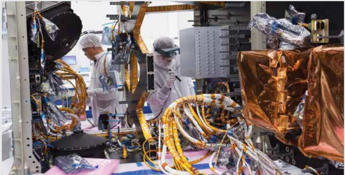
Engineers inspect the second of three RCM satellite buses in the Magellan facility. Batteries are visible in the foreground, wrapped in thermal blankets. A reaction wheel is on the left. (2016-02-11)
