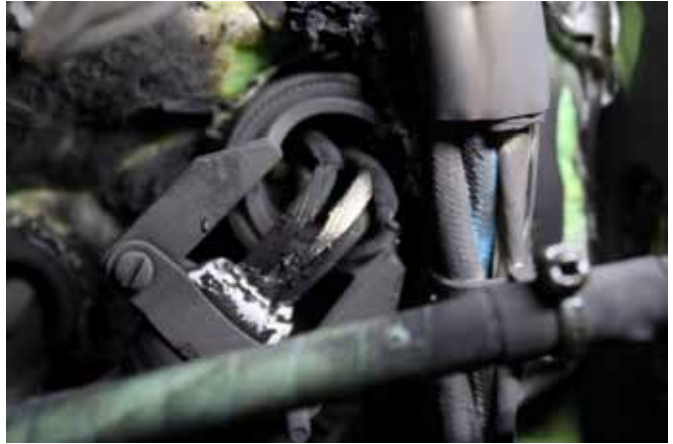
Figure 3. Electrical connector 9811-J711 on the occurrence aircraft
