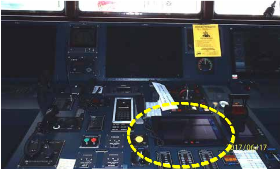
Figure 2. Centre bridge console on the Damia Desgagnés , showing the horizontal mounting location of the integrated touch screen that was activated and caused the accidental main engine shutdown
