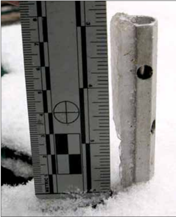
Figure 6. Ice on the right side of the vertical stabilizer
