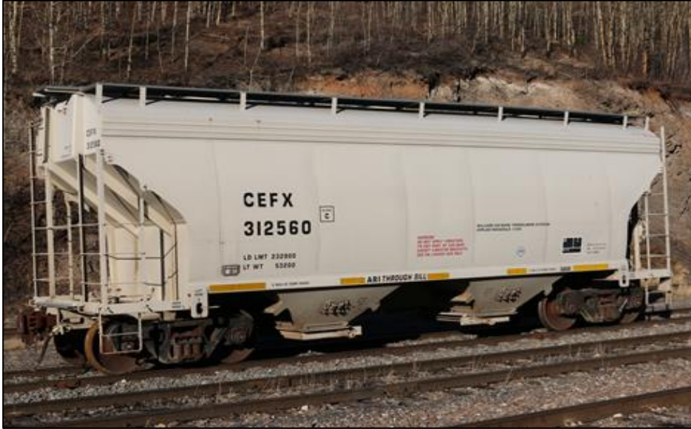
Figure 4. A typical 42-foot covered hopper car
