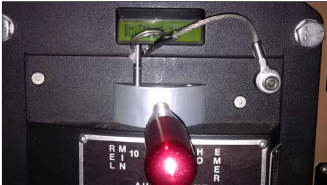
Figure 4. Automatic brake handle with locking pin inserted into the hole on the left side of the base of the handle, preventing the brake from being released.
