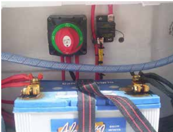
Figure 2. Builder-approved and standard battery bank arrangement in both battery compartments (Source: LeisureCAT Australia, LeisureCat 8000 Sportsfisher Owners Manual )
