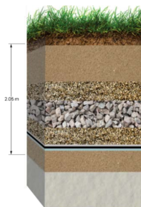
Figure K.12: Artist's rendering of closed and capped near-surface disposal facility along with liner system detail, as proposed to be constructed at Chalk River Laboratories
