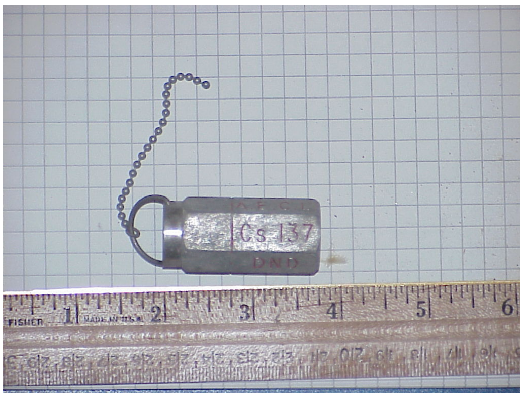
Figure J.1: Cesium-137 radioactive sealed source
