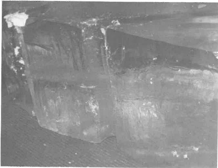
FIGURE 5. FAILED FRESH WATER ICE CYLINDER AFTER A DILATOMETER TEST.
