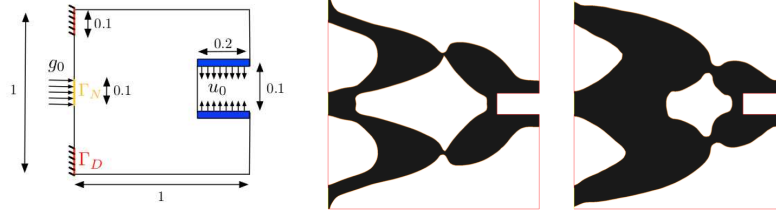
Figure 2: Gripping mechanism: loadings (left), unperturbed optimal design (middle), linearized worst-case design (right).
