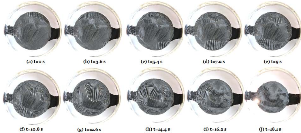
Fig. 3 The membrane of a dielectric elastomer exhibits discontinuous phase transition from the flat to wrinkled states, when voltage reaches a critical value. (a) – (j), the state of the membrane at the fixed voltage ( \Phi = 7.38\text{kV} ).
