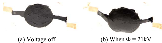
Fig. 2 Buckling of the membrane with \lambda_{pre} = 1
