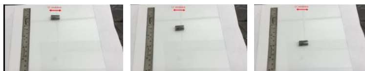
Fig. 3 Rolling of a LCE tube driven by heating.
