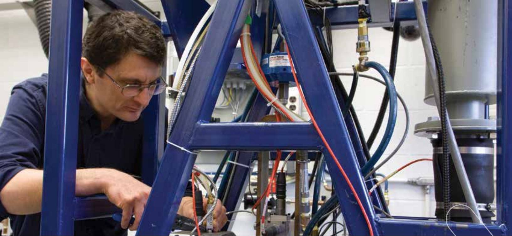
The Oil-Free Bearing Rig is used to evaluate the steady-state and dynamic characteristics of foil bearings.
