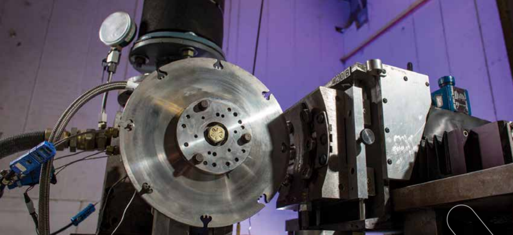
The Abradable Seal Rig simulates operational wear using a bladed disc and a test coupon fixed to a motion table.
