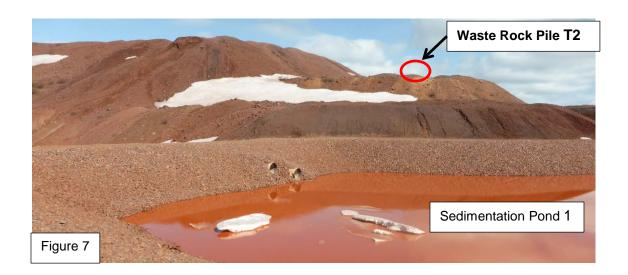
Sample **Waste Rock Pile T2** is composed of silty sand with angular gravel, loose but relatively dense. According to the Munsell Soil Colour Chart, the colour of the material is Dark Reddish Brown (2.5 YR 3/4), associated to iron oxides.
