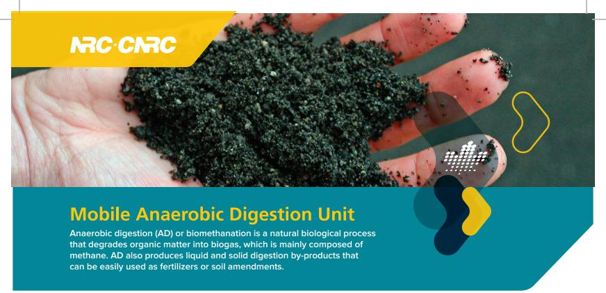
The NRC mobile AD unit is designed to demonstrate the potential of anaerobic digestion for treating wastewater, sludge and other organic material to engineering firms and their industrial or municipal clients seeking to reduce the organic load in effluents as well as associated costs. Performance data gathered during an on-site trial — i.e. volatile solids (VS) reduction, methane production and processing rates — can subsequently be used to scale up the process.
