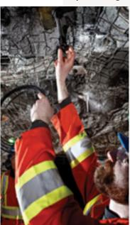
tation of microseismic monitoring systems has significantly advanced the ability to improve mine safety by providing real-time decision-making information regarding re-entry, seismic hazards, and planning. The NRC's RBS™ allows large scale cost effective deployment of this technology as sensors have low fabrication and maintenance costs, robustness of assembly, and are easy to install. Benefits of the technology are further enhanced by providing wireless options and real-time access to data.
