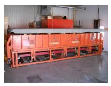
Figure 3: NRC's table for dynamic uplift resistance testing
