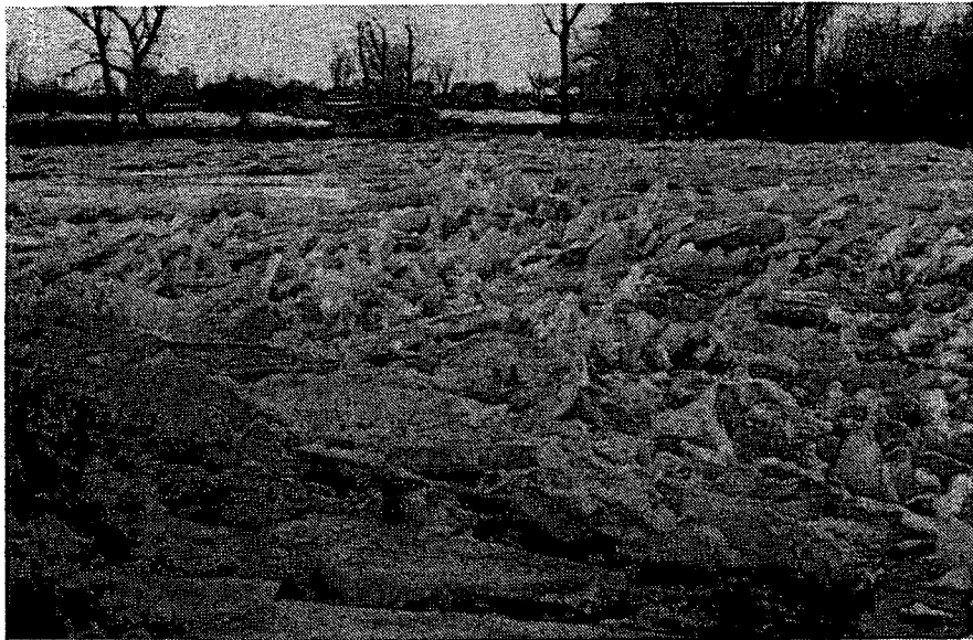
Photo 2. →d/s, 0840, 23.01.86 Surface appearance of jam near toe.
