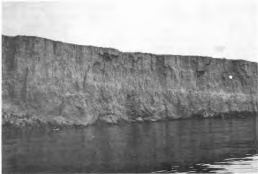
Figure 11. More advanced cliff formation. Note columnar jointing in till, resulting from desiccation; wet zone at base of cliff not fully drained. Height of cliff is approximately 11 feet. East bank of Diefenbaker Lake north of Riverhurst Ferry. August 16, 1966.
