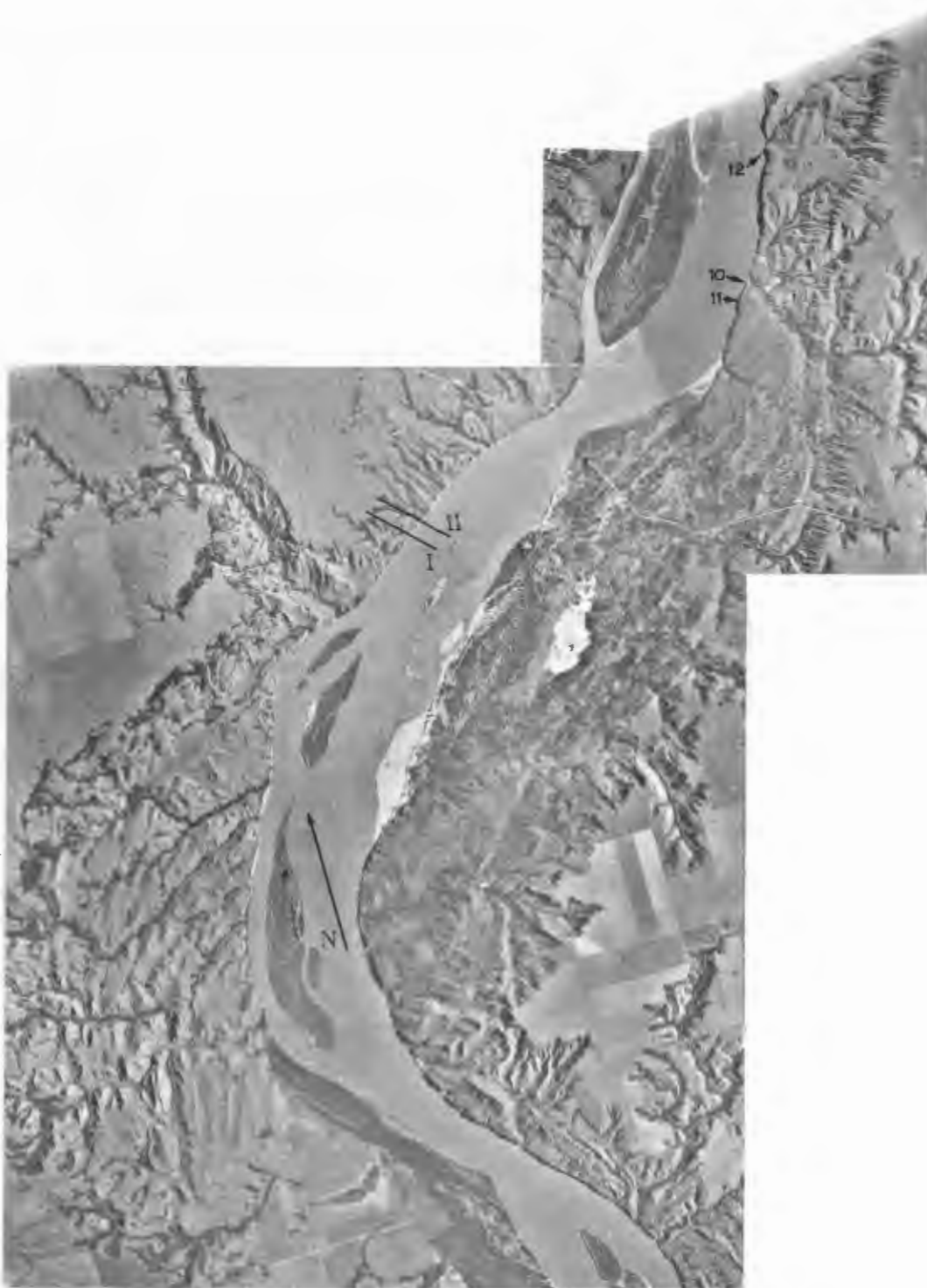
Figure 2. Valley of South Saskatchewan River near Riverhurst Ferry, Saskatchewan. Note evidence of earlier landslides mainly on west bank; and sandy area on east bank inside main bend. Numbers refer to location of photographs Figures 10 to 12; arrows indicate direction of view; Roman numerals indicate sections of Figure 17. (RCAF - A15963-121/123)
