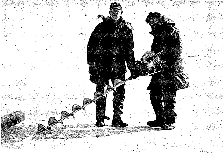
Figure 5. Powered drill fitted with a long auger shaft.
