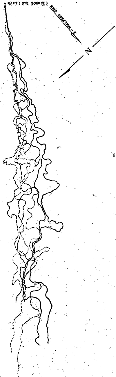
Figure 25. Dye plumes at different times, September 9, 1968. (Flight No. RC 3)
