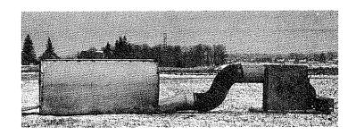
Oil Recovery International has recently introduced the SHARK 5000, a heavy oil recovery unit which uses a chain-link belt to recover viscous oil at rates claimed to be as much as 30 tonnes per hour. The unit is powered by a 2-cylinder air-cooled diesel engine. For further information contact: Oil Recovery International, Tuckton Bridge, Christchurch, Dorset BH23 1J5, England, phone (0202) 486666.
