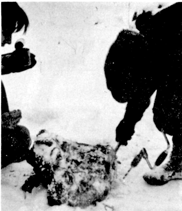
Fig. 6. Tamping in a pellet with a willow stick. The holes were closed with a few blows of a hammer.
