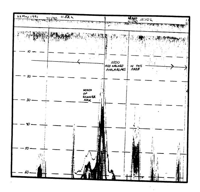
FIGURE 14. Annotated depth sounder trace from Mathieson Channel showing signals believed to be shrimp, 23 May 1991.
