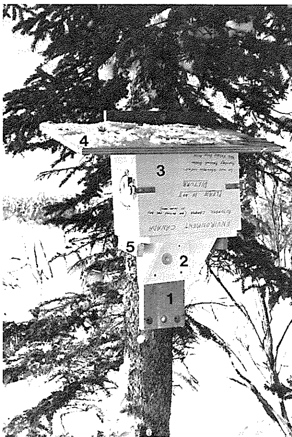
Figure 10. Camera housing installed: 1—sub base; 2—shelf; 3—housing; 4—roof; 5—braces.
