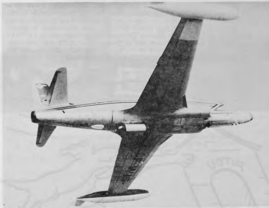
National Aeronautical Establishment T-33 Aircraft with Seed Flare Rack on Underside.
