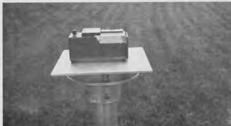
A close-up of the sunphotometer on its stand.
