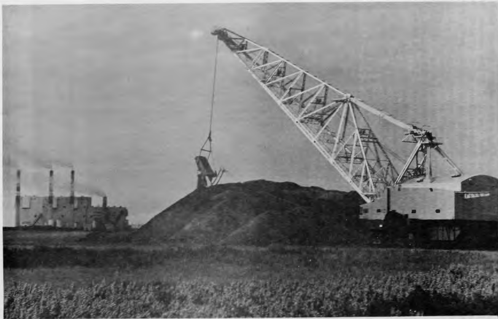
Dragline with 40 cubic yard bucket stripping overburden from coal only a mile from the Weather Office—the power plant that uses the coal to produce steam is seen in the background.
