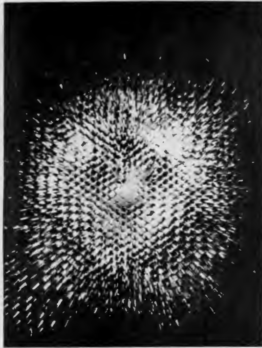
Looking into the tunnel through a honeycomb grid at the intake. The honeycomb is used to smooth the airflow entering the tunnel.
