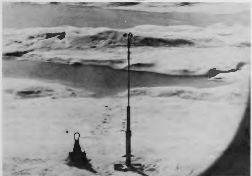
As the CANMAR helicopter lifted off from the ice floe, Bill Hart photographed the newly installed floating automatic weather station and the location device to its left.
