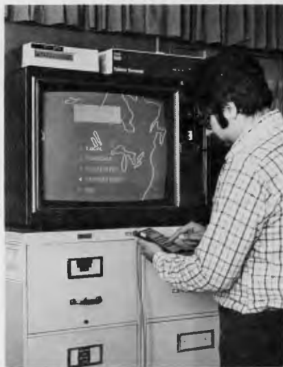
Tom Ostry uses Telidon equipment to demonstrate the weather information stored in the central computer. After having ordered the weather page, he selects from one of five choices by pushing a number on a device which resembles a calculator.
