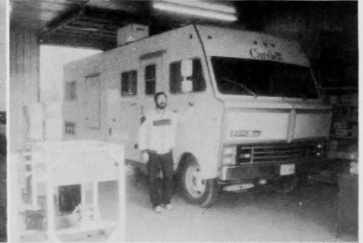
Equally farm-conscious are scientist from the Atmospheric Dispersion Division. This truck is fully equipped to do atmospheric probing of aerosol structures in the boundary layer. Standing beside the vehicle is F. Froude, electronics technician.
