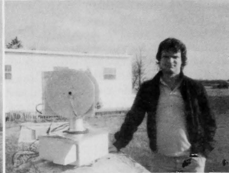
Still very active, however, is this solar radiation suntracker operated here by technician David Barton of Experimental Studies Division.
