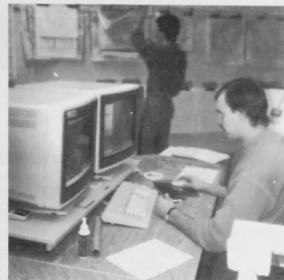
Jacques Colin keys in vital information at an Ice Data Integration and Analysis System (IDIAS) work station. The multi-computer system obtains ice data from many sources and creates sophisticated, accurate, on-screen maps.
