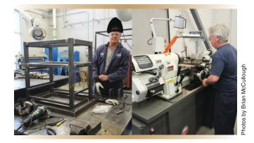
The facility's enhanced welding and machine shops are equipped to manufacture and set up the unique test rigs needed for shock and vibration testing, environmental testing, pressure testing, or whatever else is required.
