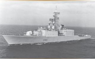
The Tribal-class Update and Modernization Program of the mid-1990s replaced the distinctive V-mounted "bunny ear" funnels with a single uptake, and mounted a 76-mm gun in place of the 5"54-calibre gun and Sea Sparrow missile housing on the fo'c'sle.
