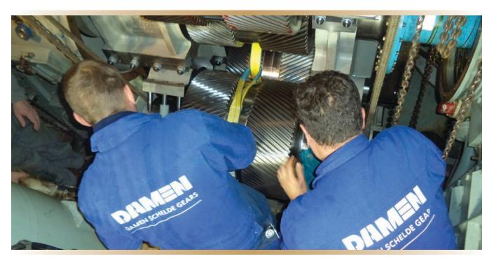
Figure 8. Idler gear being installed in the gearbox.
