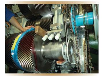
Figure 6. Idler gear being rolled out of the gearbox.
