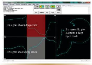
6 ACFM measurement of Crack #1 Flank
