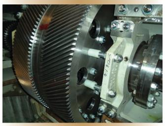
Figure 7. Gearwheel fitted with temporary brakes (white plastic).
