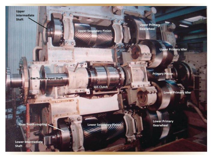
Figure 5. Starboard gearbox.
