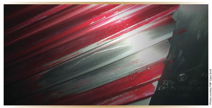
Figure 1. Surface crack shown during initial gear inspection.
