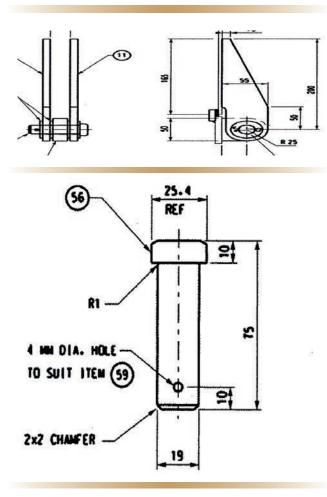
Figure 4. Schematics of the hinge and hinge pin.
