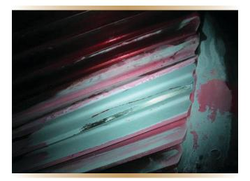
Figure 2. Surface crack shown by liquid penetrant testing.
