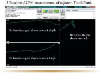
Figure 3. ACFM inspection of a normal tooth.
