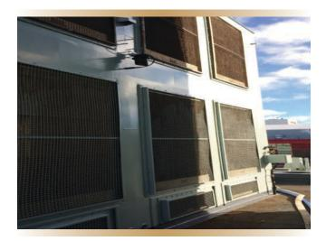
Figure 1. The gas-turbine air intakes on the upper deck of a *Halifax*-class frigate.
