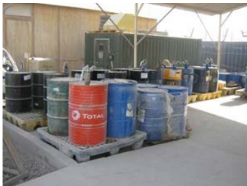
Figure 3: Combined Secondary Containment for HAZMAT
