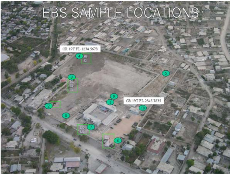
Figure 1: Example Environmental Baseline Study Sampling Locations Annotated with Military Grid Reference System Coordinates
