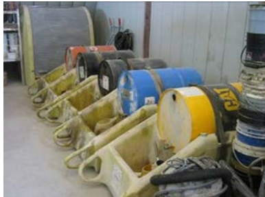
Figure 4: Separate Secondary Containment Dykes for HAZMAT
