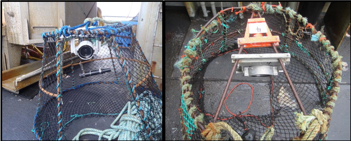
Figure 2. A) Camera in bracket. B) Front view (left) and top view (right) of camera (grey bracket) and accelerometer (orange bracket) mounted in Sablefish trap.
