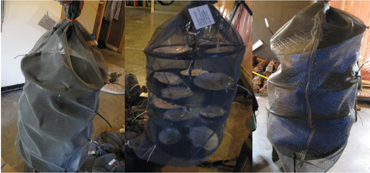
a) b) c) Figure 4. Suspended experimental collectors a) No substrate b) Scallop shell substrate c) Netron™ substrate.
