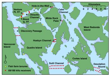
Figure 44-3. Map of the acoustic receiver array used to track juvenile salmon through the Discovery Islands and near salmon farms in 2017. Yellow lines and dots represent single frequency (69 kHz) receiver sub-arrays, while red dots and lines represent dual frequency (180 kHz) sub-arrays. Discovery Passage, Sutil Channel, and Desolation Sound were deployed 2015-2017, while Hoskyn and Okisollo channels were only deployed in 2017.
