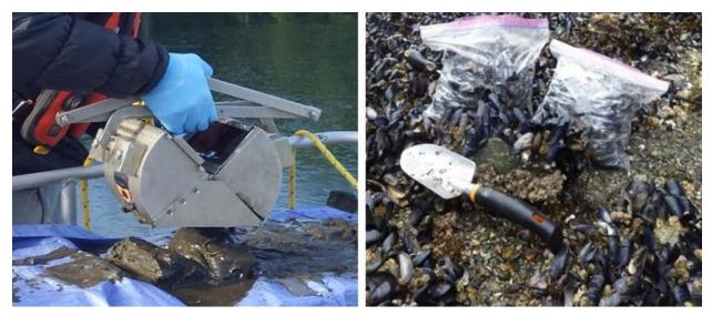
Figure 30-2. Sediment samples are collected using a petite ponar grab (left), while mussel samples are collected by hand (right).
