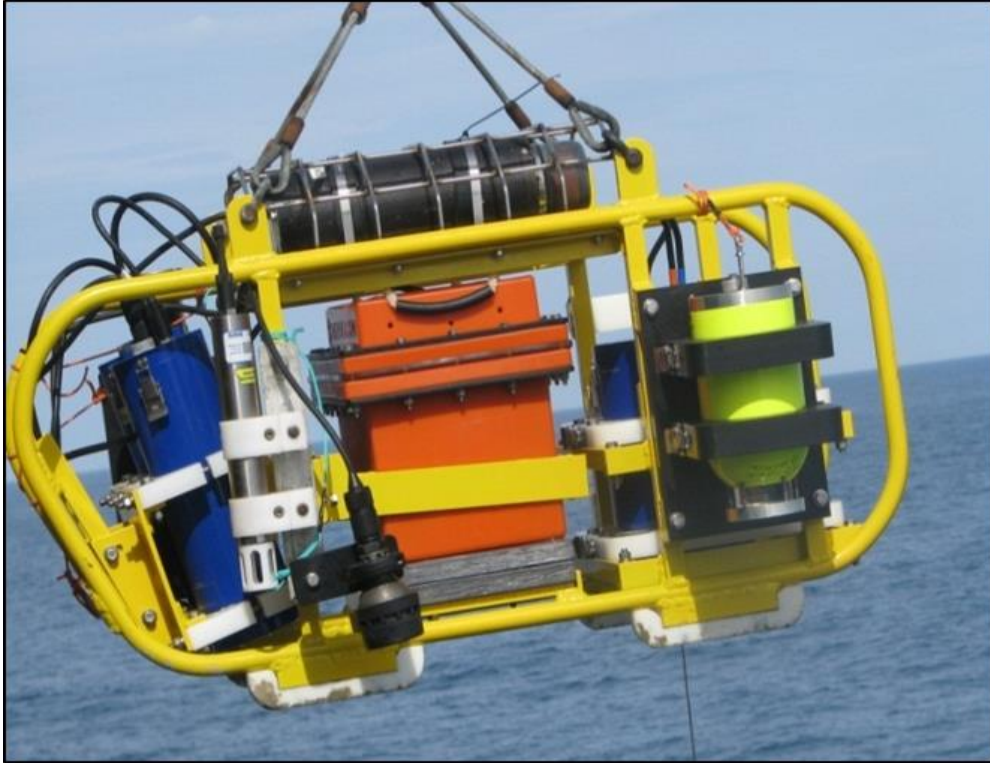
Figure 2. The 4KCamera drop camera system being deployed to collect Arctic images.
