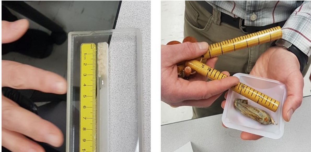
Figure 5. Tools used to estimate prey volume at-sea: left: the King-Zubkowski volume measuring trench used by pelagic ecosystem surveys at the Pacific Biological Station; right: the Food Web Dynamics Program (FWDP) at the Northeast Fisheries Science Center uses 'wind chimes' for prey volume estimation.
