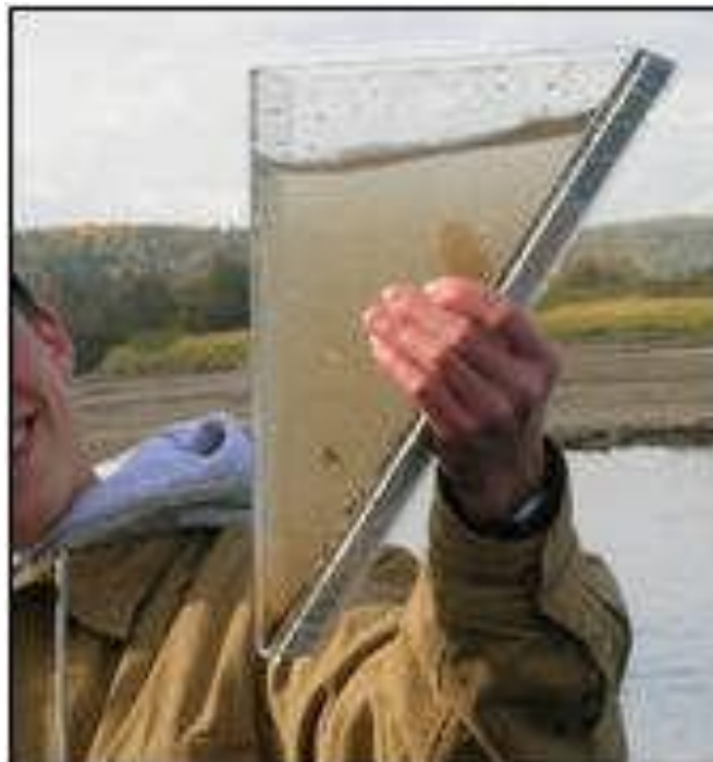
Turbidity Wedge – used to determine how muddy the water is
