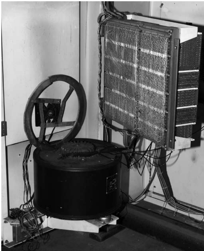
Figure 23: UMAC-5 transistor/drum memory. (CSTM 1985.0359.001)
