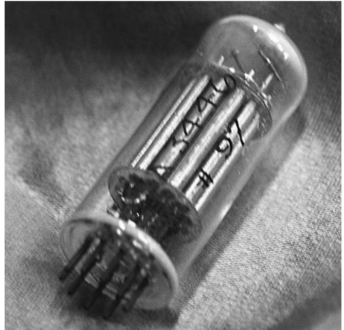
Figure 5: Joseph Kates’s binary adder tube known as the Additron. (CSTM 1990.0221.001)
