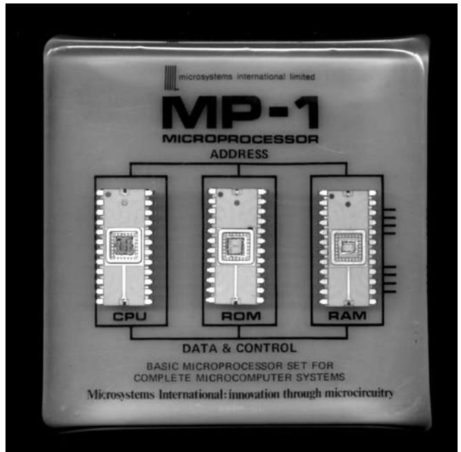
Figure 31: The MIL MP-1 chip set, consisting of the MF7114 CPU, the MF1601 ROM and the MF7115 RAM. Image of MIL's MP-1 promotional paperweight. (Courtesy York University Computer Museum)
