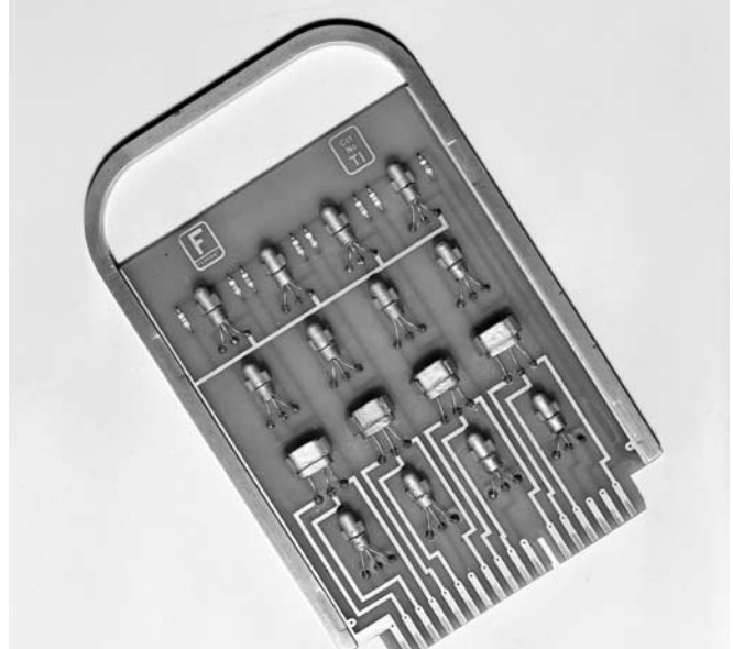
Figure 14: Mail-sorting computer, transistor board, 1955. [Courtesy Archives of Ontario, Ferranti-Packard Collection, subseries F-4142-12-5-1, container A-1080, image 1093]
