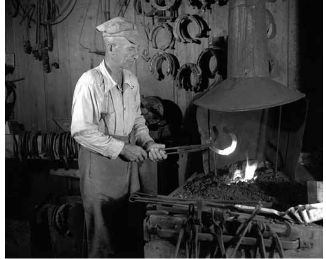
Figure 2.7: Blacksmiths like Joseph-Louis Paquet continued using the heat of the forge to alter horseshoes, Saint-Côme, Quebec, 1952 (Photo by Omer Beaudoin, BANQ, E6, S7, SS1, P92908)
