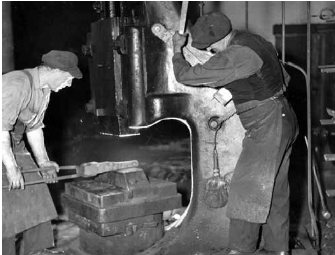
Figure 3.11: Flattening an iron bar with a mechanical drop-hammer, Port Mann, British Columbia, 1948 [CSTM, CN Collection, #761]
