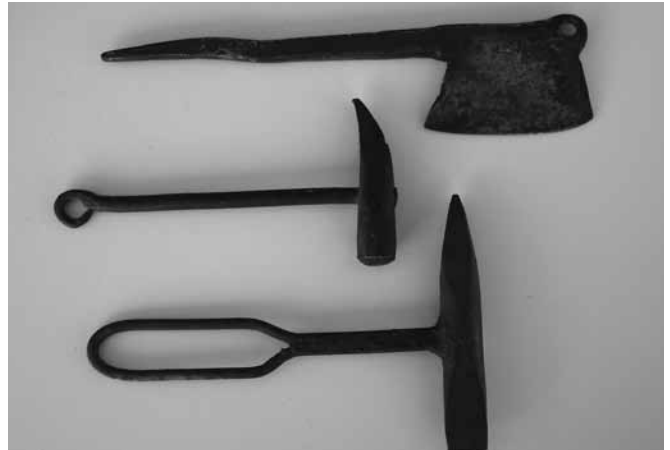
b) butcher's cleaver, carriage snow hammer and multi-purpose hammer (Photo by author, DTR)
