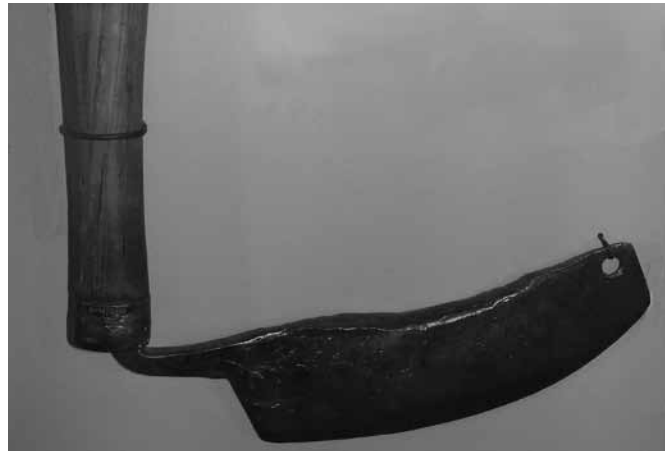
d) froe used to split shingles (NSM)
