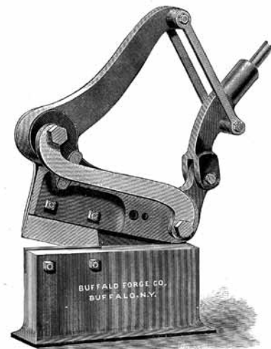
Figure 3.15: Continuous shearing machine used by blacksmiths during the nineteenth century [CSTM, Trade Lit.: Buffalo Forge Co., Illustrated Catalogue , Buffalo, N.Y., 1896, p.326]
