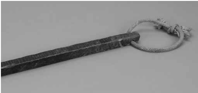
Figure 3.6: Nose twister used in the nineteenth century to quiet a restless horse while it was being shod, Portneuf, Quebec (CMC, D2007-7201)
