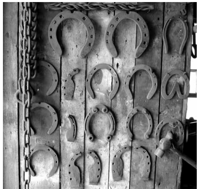
Figure 4.6 Horseshoes with iron cleats and caulks added to prevent slipping (Photo by author, DTR)
