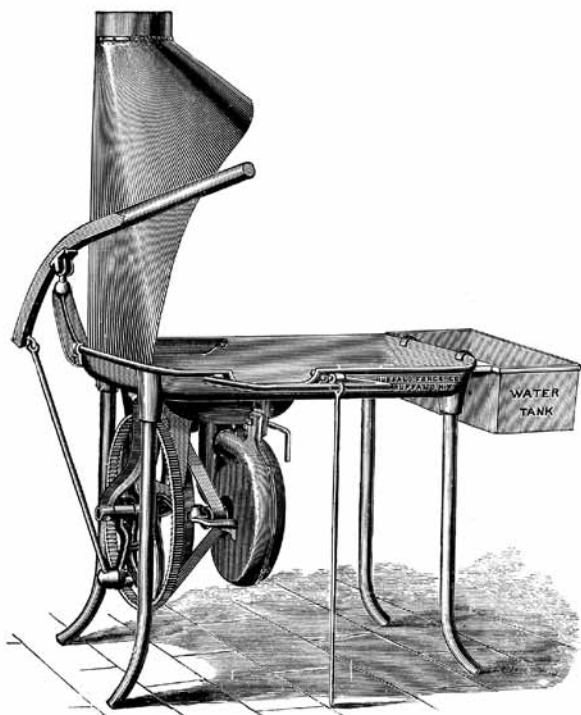
Figure 3.8: Portable forge: standard model employed by blacksmiths, late nineteenth century (CSTM, Trade Lit.: Buffalo Forge Co., Illustrated General Catalogue , Buffalo, 1896, p.294)
