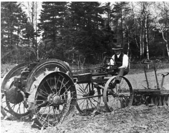
Figure 1: The early gas-powered front-wheel-drive Moline tractor was a symbol of more important machines to come (Prince Edward Island Archives, P-2708)
