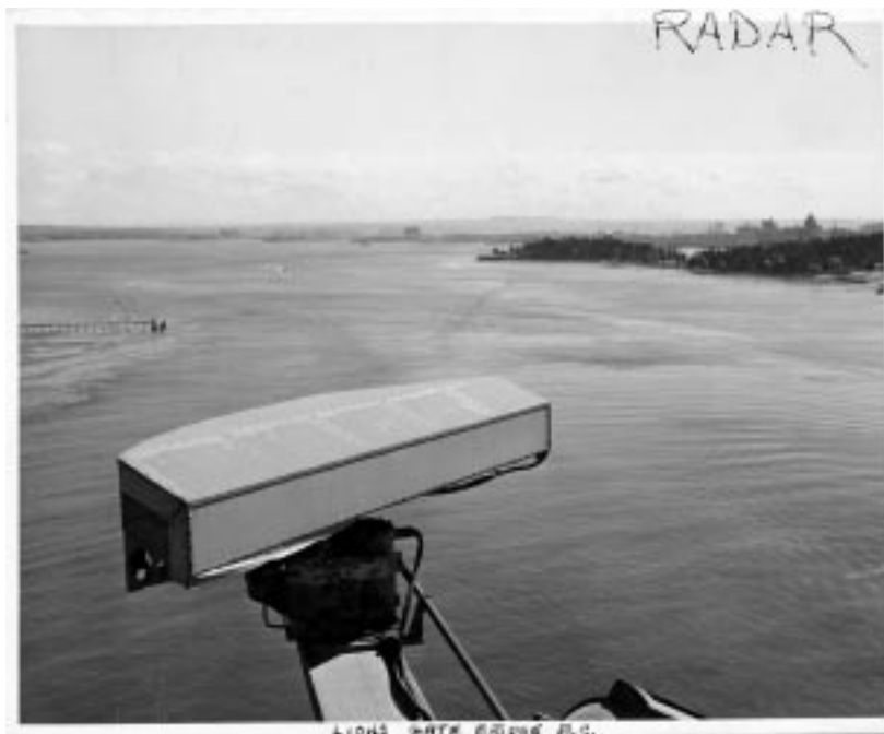
Figure 65. Canadian officials began experimenting with harbour radar in the late 1940s, setting up systems at Camperdown, Nova Scotia, in 1946–47 and the following year on the Lions Gate Bridge in Vancouver, shown here. These systems were a precursor to the more elaborate vessel traffic systems established in the late 1960s.
