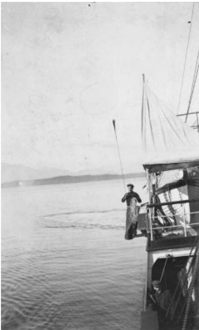
Figure 43. GGS Quadra around 1900. Before the advent of sonar in the 1930s, mariners and hydrographers measured the water's depth and mapped the sea bottom using a lead line like the one in this photograph. This ancient tool had changed little over the course of many centuries.
