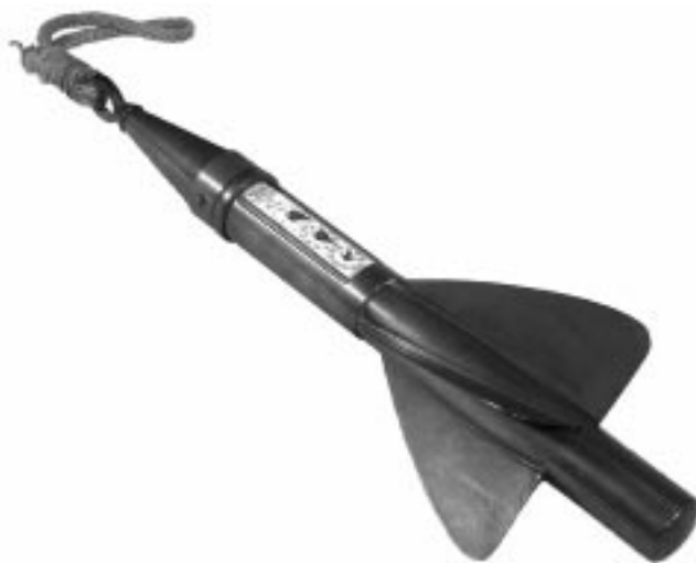
Figure 22. This taffrail log was manufactured by Thomas Walker probably around the mid-nineteenth century. Known as a harpoon log, it was one of many that incorporated improvements on the first mechanical log introduced by Edward Massey, Walker's uncle, in 1802. (CSTM1977.0392)
