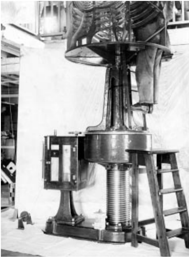
Figure 50. Adoption of high-power electrical lights made it possible to replace many of the large, expensive, and high-maintenance Fresnel lenses. This image shows a staff member working on the third-order Fresnel apparatus from the Point Ferolle light.
