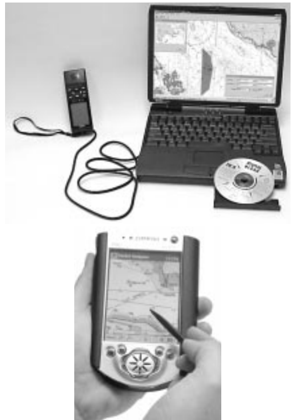
Figure 47. Detail of an electronic chart showing the ship’s course, direction and speed. Note the larger chart from which the detail is derived in the upper left-hand window. Though most ships equipped with ECDIS would have a built-in monitor and processor, navigators can also use portable devices like the two shown here to link into the ship’s navigational systems.
