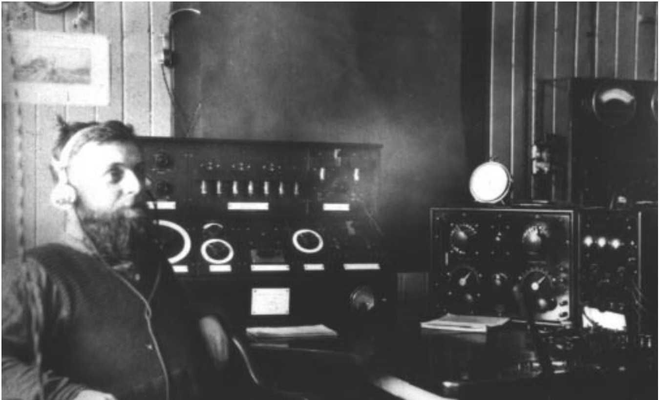
Figure 40. Alexander “Sandy” McLean at Canadian government marine radio station VCM Belle Isle, Newfoundland, winter 1925. McLean sits in front of a Marconi direction finding set. Next to the DF set is a receiver used for conventional radio communication.
