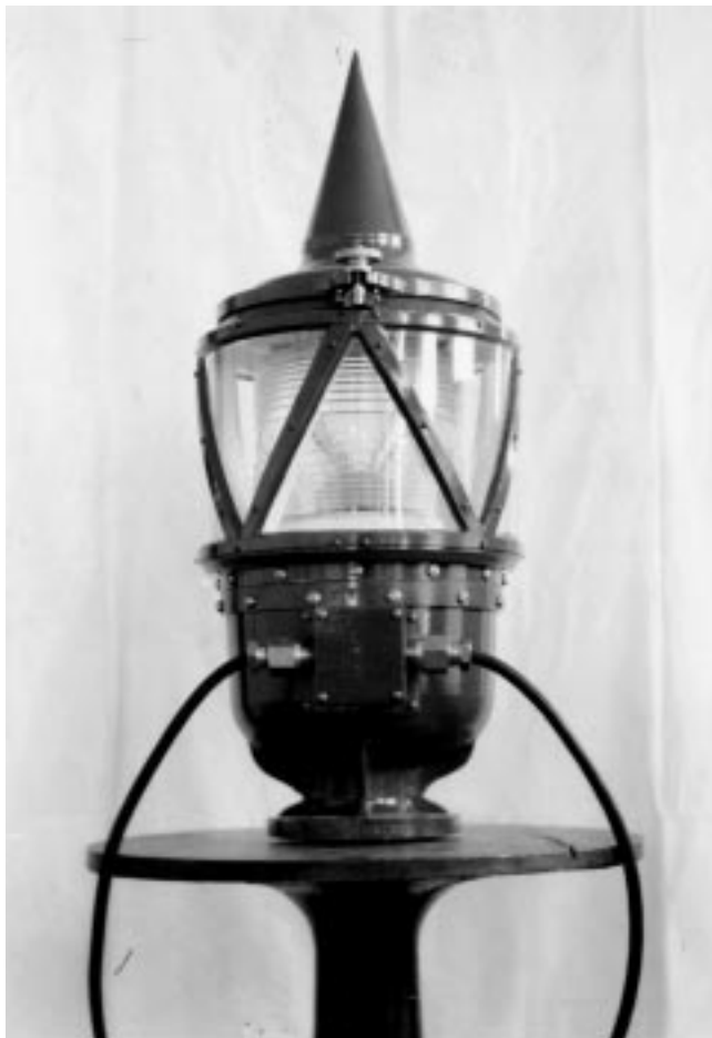
Figure 49. Canadian marine authorities began to install electric lights in their navigational aids around the time of the First World War. This particular lamp probably dates from after the Second World War, and included a sun valve that automatically turned the light on when the sky got dark.
