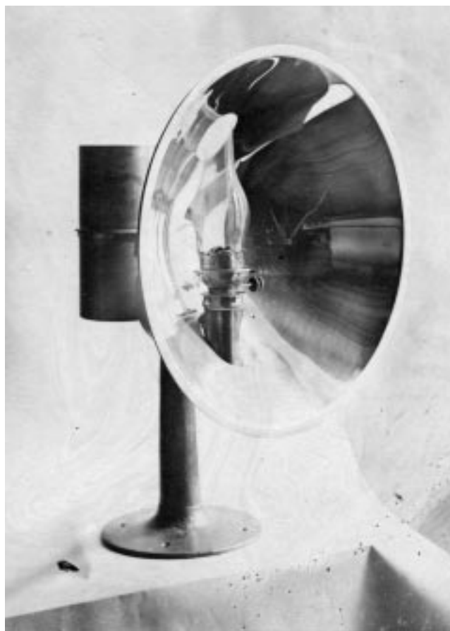
Figure 26. This wick-type lantern and 24-inch reflector were the front part of a range marker. Ranges consisted of two lights that, when lined up by a ship's navigator, indicated a safe course.
