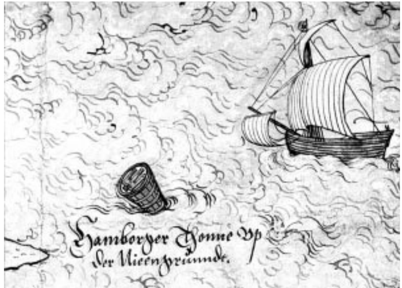
Figures 13 and 14. Late-sixteenth-century conical barrel buoy with its mooring chain linked at the narrow end floats upright in the water.
