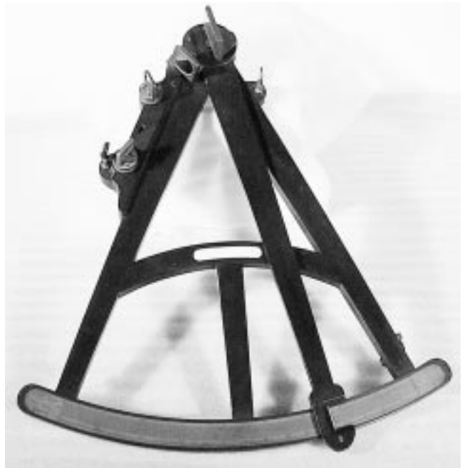
Figure 6. A Hadley’s octant manufactured between 1766 and 1782 by English maker Benjamin Cole Jr. The large-radius octant was gradually replaced by the small-radius models made possible by the introduction of mechanical dividing engines. This instrument was owned by a Canadian, G. C. Morrison of Glenholm, Nova Scotia. (CSTM1992.1569)
