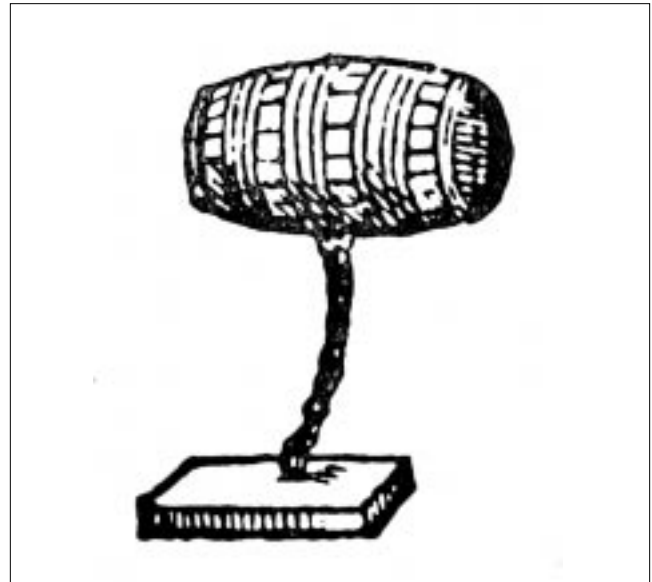
Figure 12. A simple barrel buoy of the late sixteenth century. This type of buoy, with its symmetrical shape and mooring chain attached to the centre of the barrel, lies flat in the water.
