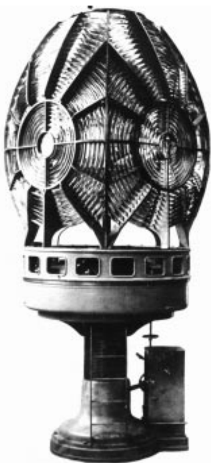
Figure 27. First-order Fresnel lens and single flashing apparatus, Langara Island light, B.C. (Library and Archives Canada, neg. PA 121757)
