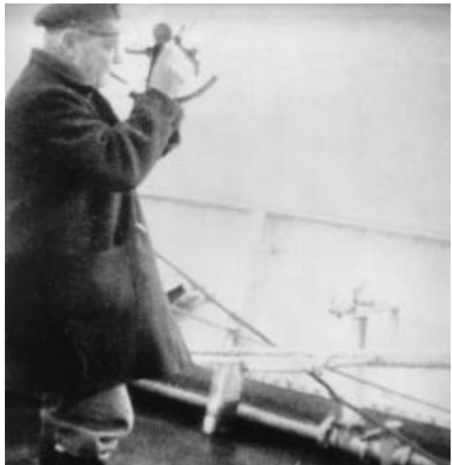
Figure 7. The captain of the Finnish barque Passat circa 1947 using a sextant. Invented in the mid-eighteenth century, the sextant became and remained the primary tool for establishing latitude on board ships for more than two hundred years. (Courtesy Niels Jannasch)
