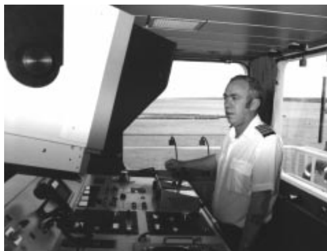
Figure 45. Control console of the MV Caribou showing PINS video display terminal in left foreground. (Offshore Systems Limited, Vancouver, no neg. no.)
