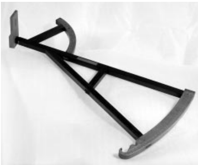
Figure 5. The back-staff or Davis quadrant was invented by John Davis around 1590 and served mariners well for over 150 years until it was gradually supplanted by the octant. This one was made by John Cranevelt of the Netherlands between 1725 and 1775 of mahogany and boxwood. (CSTM1992.0038)
