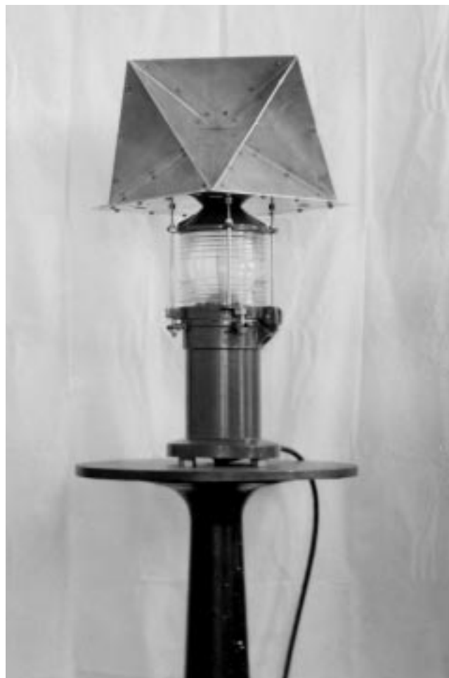
Figure 64. After 1945, Canadian marine authorities began to incorporate radar into their aids to navigation. This light-weight electric lantern has a radar reflector attached to it, allowing radar-equipped vessels to “see” the seamark to which it was attached even in foggy conditions.
