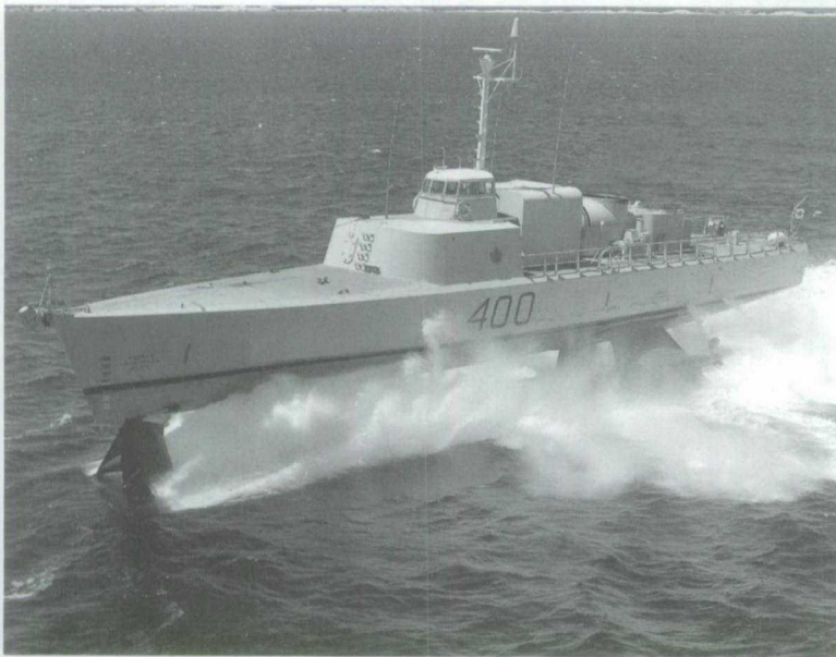
The FHE-400 naval hydrofoil, foilborne. (Courtesy of de Havilland Canada).
