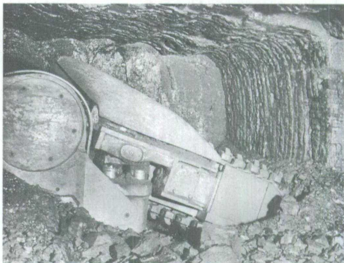
DOSCO Miner in action, DOSCO No. 18 colliery, 1953. Most of the technology applied to Canadian coal mining was transferred and adapted from outside. The British influence had been superseded by the American in the course of the 20th century. After World War II, it was apparent that a major technological push was required if the price of Nova Scotia coal was to be competitive with the American product. The DOSCO Miner was an attempt to meet the needs of the local community with a uniquely designed automatic miner that was developed within Canada. In reality, the DOSCO Miner was an adaptation of mobile cutting machines that had been in evolution in the U.S. for the previous two decades. It took the components of the machinery — most of it from the Joy Manufacturing Company of Cleveland — and designed and assembled the machines in the DOSCO factory at Trenton. After a great deal of experimentation and considerable expenditure of money, it was widely applied across the Nova Scotia industry throughout the 1950s and 1960s, though it was subsequently replaced by more advanced machinery from Europe. (Courtesy of the Beaton Institute, University College of Cape Breton).
