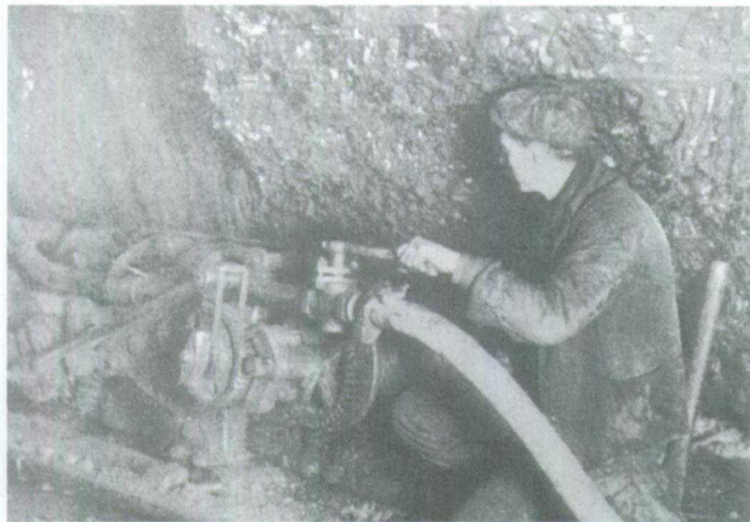
Miner operating punching undercutting machine, ca 1900. The introduction of mechanical cutters marked a change in the organization of work underground. Perhaps most important, apart from the ease with which previous hand work could now be done, was the necessity to deliver power to hundreds of places underground. Large compressors were developed above ground to provide compressed air to drive the machines. Miles of pipe and regulating equipment were required to deliver air to miners' working places, an investment that demanded much higher levels of productivity if the mine was to be profitable. Once established, such systems were prone to breakdowns, a source of constant complaint from the miners, whose earnings were directly tied to their productivity. (Courtesy of the Beaton Institute, University College of Cape Breton).
