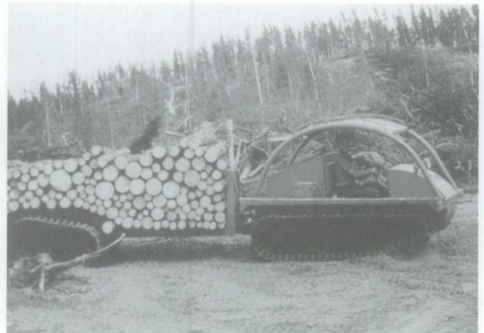
Figure 1.17 Bombardier J-5 snowmobile forwarding four-foot wood with trailer.
