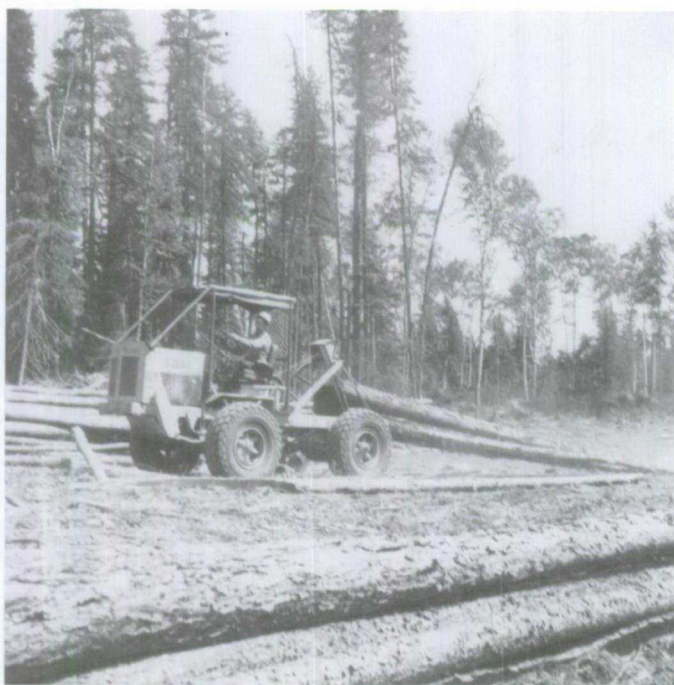
Figure 1.38 A Blue Ox skidder arriving at the landing with a load of jackpine tree lengths, 1953.
