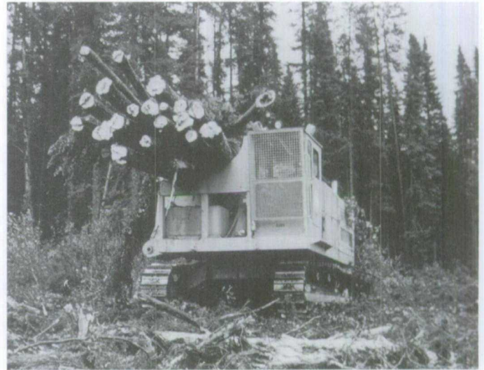
Figure 1.98 The Larson L-11 forwarding a load of tree lengths.
