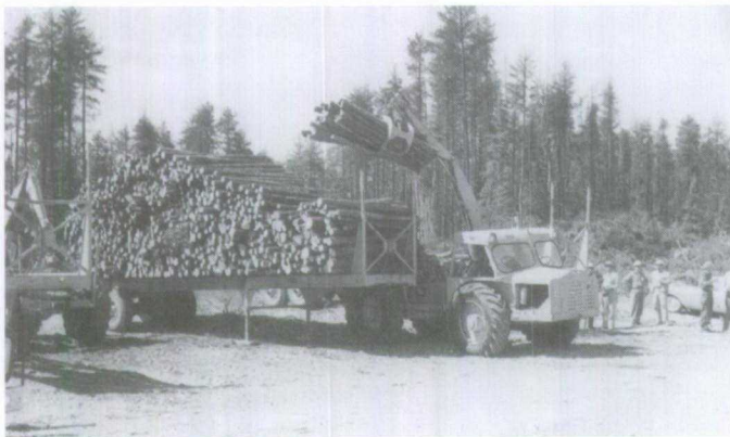
Figure 1.42 A Bonnard Forwarder off-loading eight-foot wood onto a parked semi-trailer.
