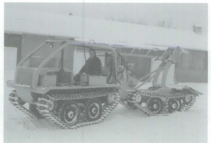
Figure 1.19 F-4 Dion snowmobile with skidding arch.
