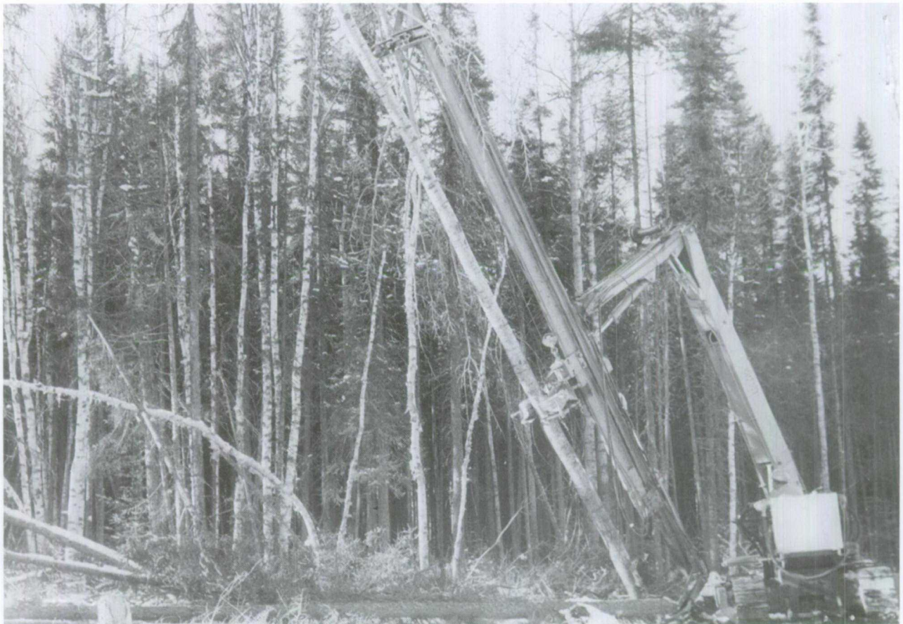
Figure 1.84 A tree being swung to the side of a Marathon Spruce Harvester to be placed in a pile.
