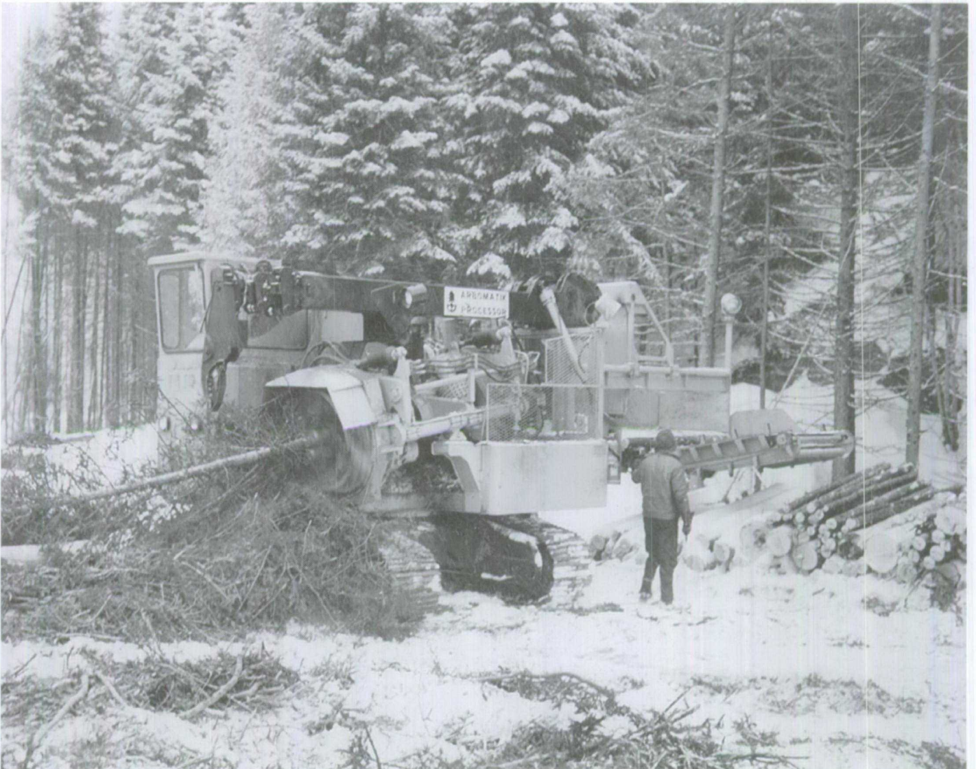
Figure 1.141 The Arbomatik Processor with discharge conveyor for piling wood.
