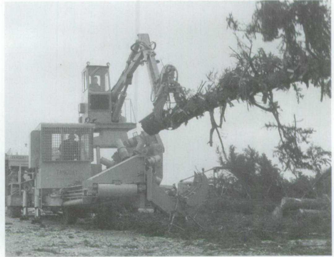
Figure 1.100 The Tanguay Slasher equipped with a Sund Delimber.
