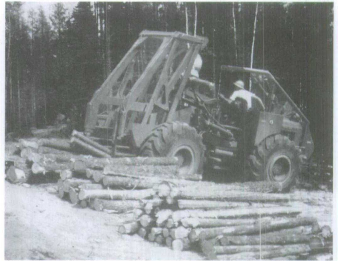
Figure 1.105 A Busch Combine piling down at the roadside.
