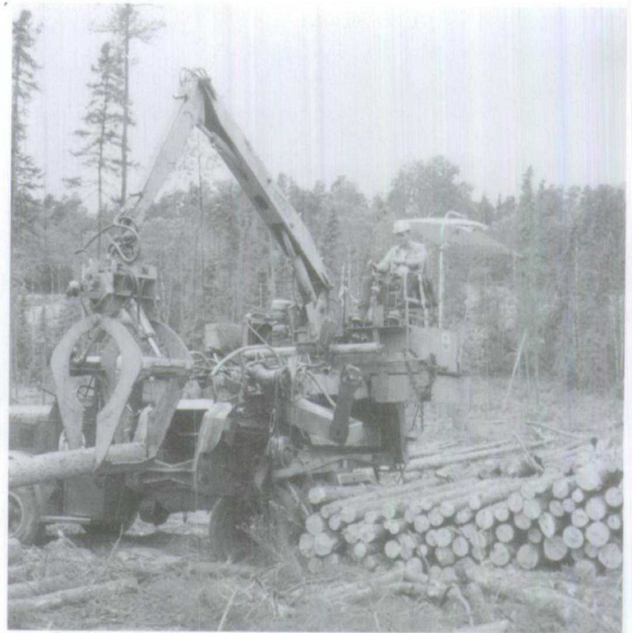
Figure 1.102 The O and M tree processor picking up a tree length by its butt and feeding it into the machine.
