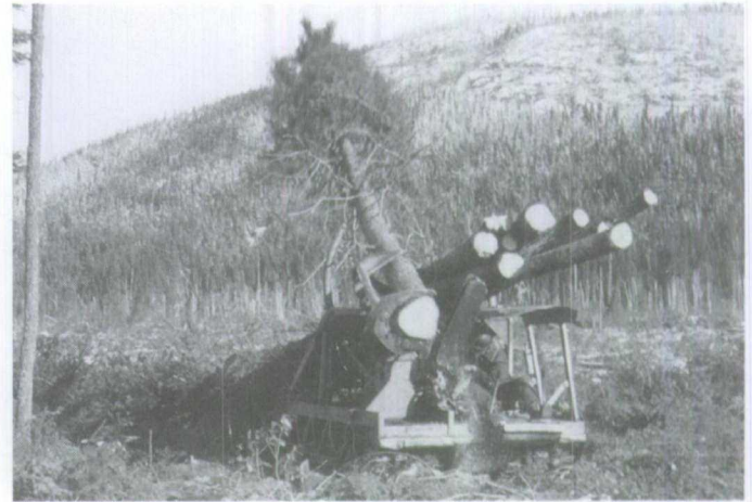
Figure 1.52 Loading a tree over top of the Vit Feller Buncher cab into the holding rack.
