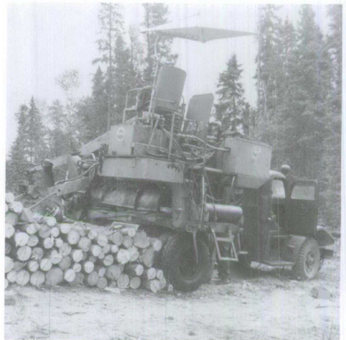
Figure 1.103 Bolts eight feet in length are discharged into the pile at the rear of the O and M tree processor.
