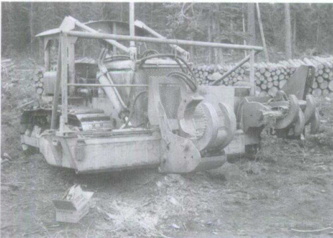
Figure 1.47 A Pope Harvester mounted on the C-frame of a D-7 tractor. The felling saw and main jaw are to the right, the delimiting jaw is in the centre. The machine approached a tree and grappled it with the main jaw, as close to the ground as possible. The tree was then severed from its stump, and held in a vertical position while the harvester moved to the chosen piling area. Then the main jaw was rotated 90°, allowing the tree to settle horizontally into the open delimiting-jaw. The arms closed around the tree and then the delimiting jaw was moved along its track, by means of a hydraulically activated cable and pulley system. All limbs were removed from the tree along the length of the track, which was 100 inches. The delimiting arms remained tightly fastened around the tree while the main clamp was opened slightly, so the tree could be pushed through by the return travel of the delimiting jaw. This action removed all remaining limbs and positioned the tree for bucking. The chainsaw had rotated to the bucking position when the main jaw had been rotated 90°. It then made the cut, and the 100-inch bolt fell to the pile (Hart 1958).
