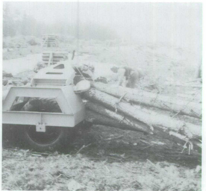
Figure 1.82 A sulky trailer, a forerunner of today's clam bunk skidder. Tree butts rest on it and are encircled and held by a scable.
