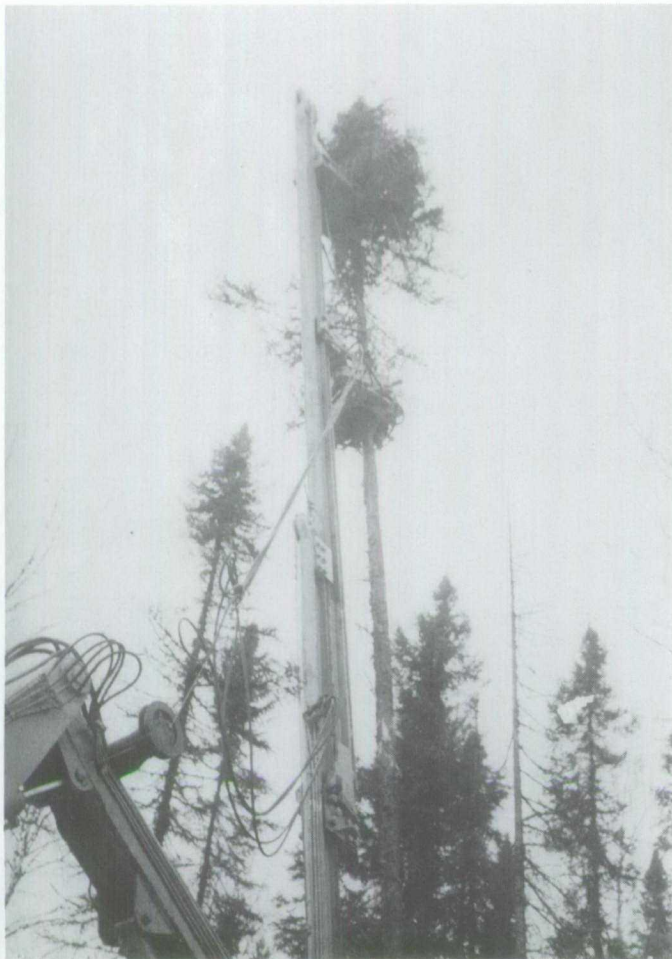
Figure 1.85 The delimiting head of a Marathon Spruce Harvester part-way up a black spruce tree. Delimiting took five seconds, shearing the top took three seconds, shearing the tree from its stump took four seconds.
