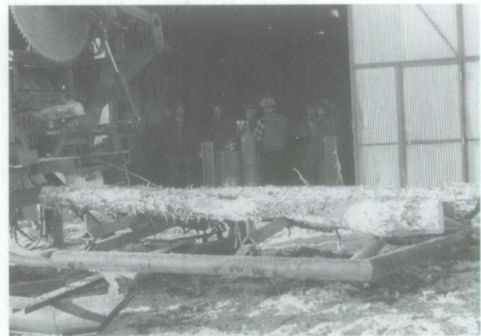
Figure 1.58 Bolts eight feet long, delimited with the chain flails of the Larson roadside processor.
