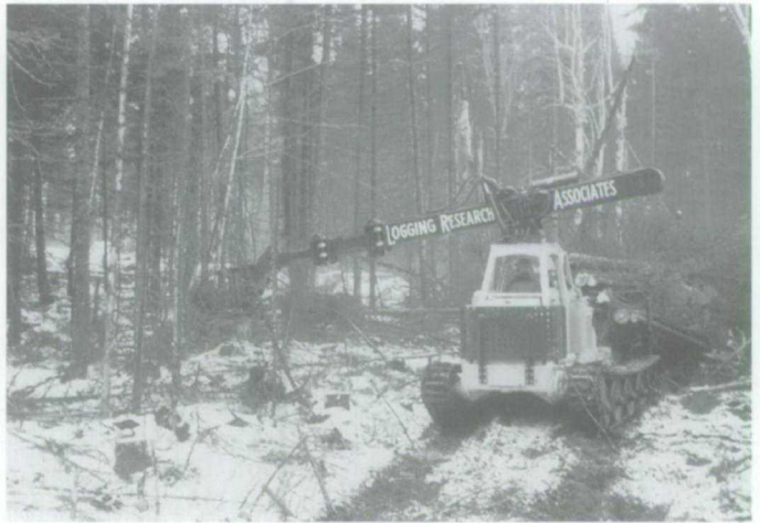
Figure 1.144 The newly designed boom eliminates the winch box and gear reducer visible on earlier booms. Roller chains instead of cables are used to activate boom sections.
