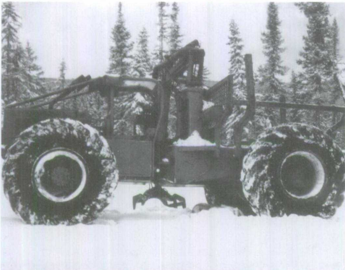
Figure 1.106 A Packjack (Timberjack Ltd) for forwarding eight-foot wood (1972).
