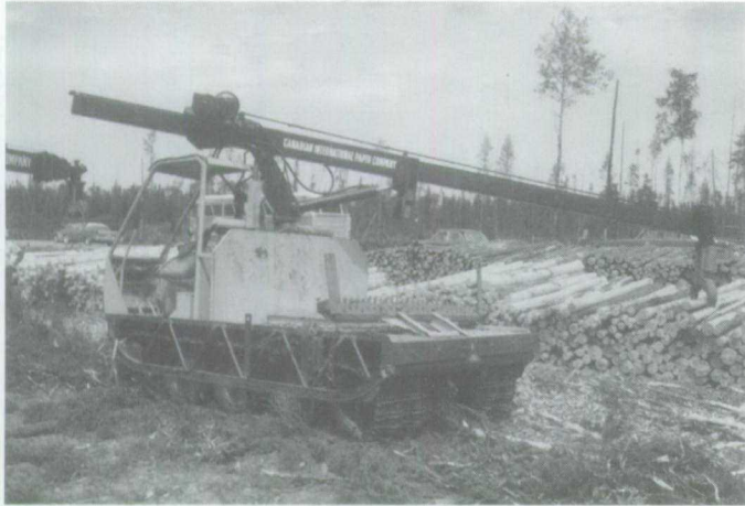
Figure 1.147 The Canadian International Paper Co. self-loading skidder on a Bombardier chassis.
