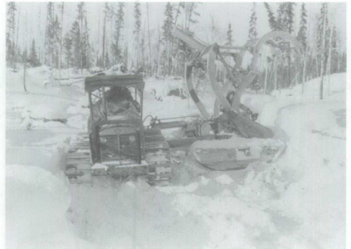
Figure 1.29 An Anderson Woodhawk (in winter) backing into a pile of eight-foot wood on a strip road.
