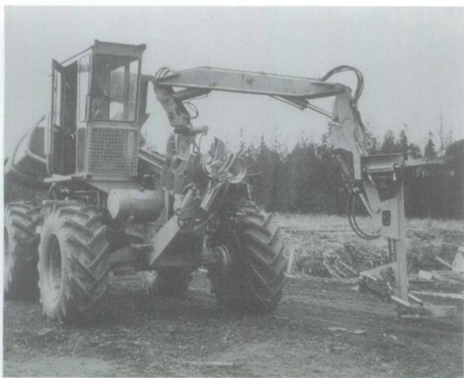
Figure 1.131 The first prototype of the Larson Shortwood Harvester had a relatively small collecting cradle.
