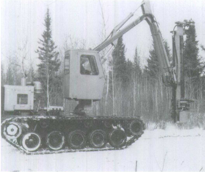
Figure 1.136 The Siiro Harvester prototype mounted on tank chassis.
