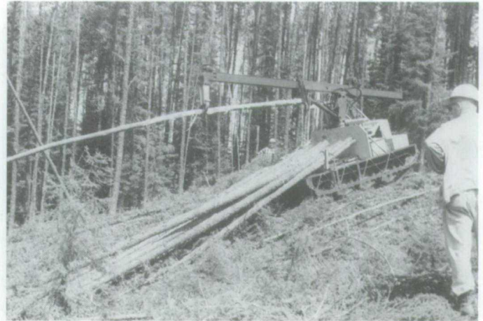
Figure 1.148 The Canadian International Paper Co. self-loading skidder in operation. A row of full trees is laid across the width of bunk and fastened, remainder of the load is simply piled on top.
