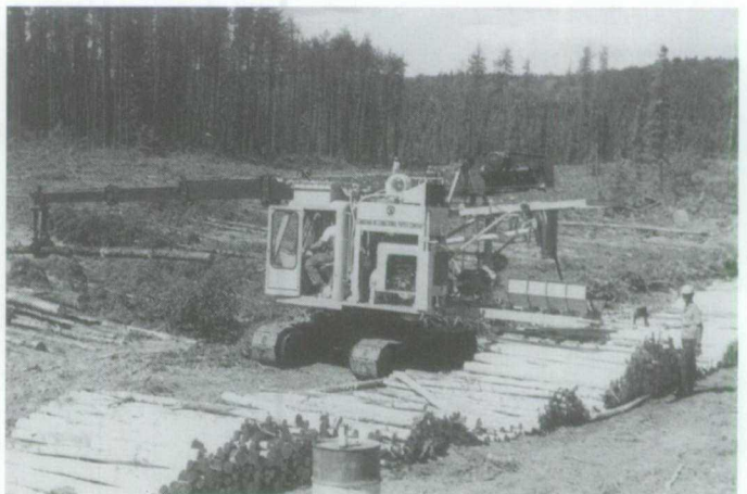
Figure 1.138 The Arbomatik Processor producing eight-foot bark-free wood.
