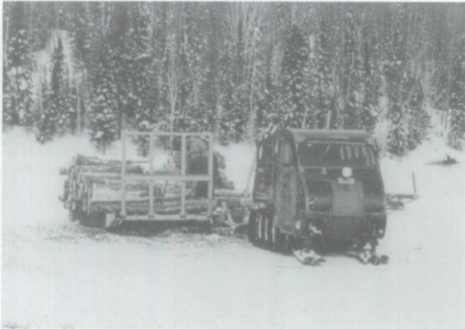
Figure 1.16 Bombardier snowmobile forwarding a single sleigh-load of four-foot wood, transferring load to truck pallet on landing.
