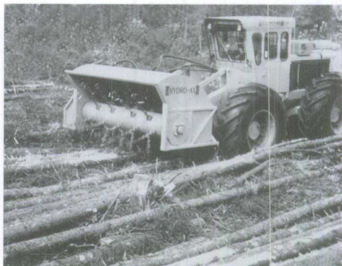
Figure 1.170 Flailing a pile of spruce trees, working from top to butt.
