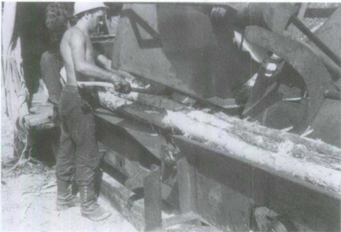
Figure 1.66 Slashing tree lengths to four-foot bolts.
