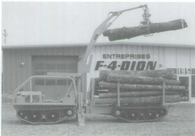
Figure 1.18 F-4 Dion snowmobile in forwarder configuration.
