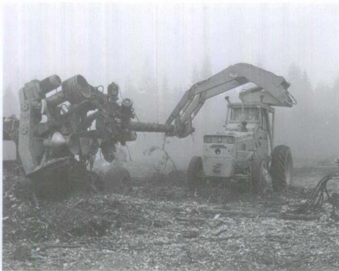
Figure 1.119 Tree feeder inserting a tree into the Sund delimiting head.
