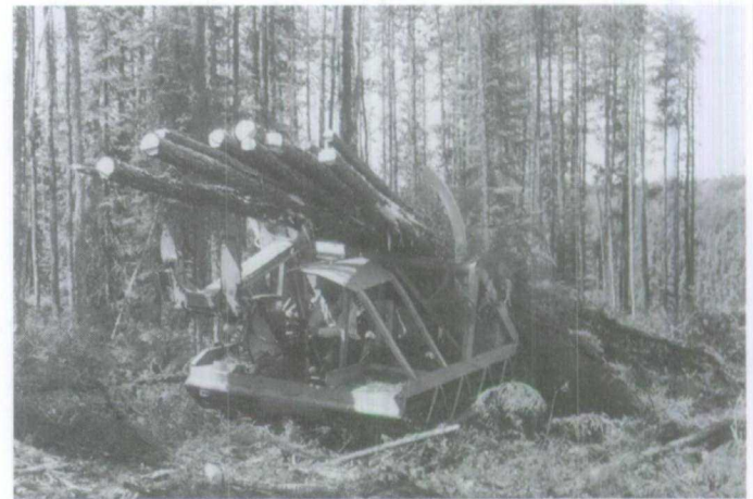
Figure 1.53 The Vit Feller Buncher moving to the next tree to be harvested.
