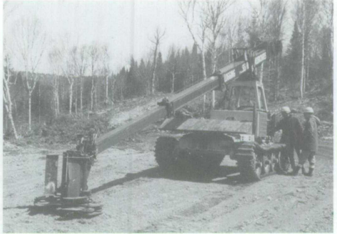
Figure 1.143 The Mark II felling head. The telescopic boom is extended to full reach (28 feet) from centre of rotation.
