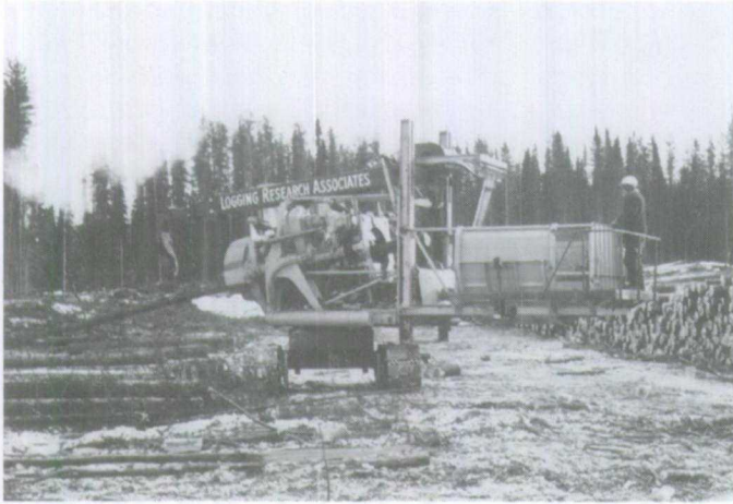
Figure 1.139 A later model of the Arbomatik Processor with large collection basket for rough wood.
