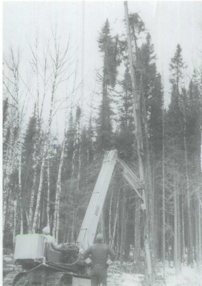
Figure 1.86 The top of the tree has been sheared by the Marathon Spruce Harvester and is falling point-downwards.
