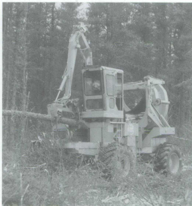
Figure 1.132 The Larson Shortwood Harvester operating in forest stand. The operating sequence for this harvester was similar to most of the others developed in this period (Bredberg 1970b). The machine moved to a position from which one or more trees would be harvested. The felling boom was extended to a tree, the felling head was positioned and the tree severed from its stump. The severed tree was lifted vertically and swung into position directly in front of the machine. The tree was lowered and held in a horizontal position until the automatic processing of the preceding tree was completed. The tree was then lowered into the open delimber and carriage arms and the automatic processing cycle started again. Simultaneously, the manually controlled felling began again. In the automated processor, the delimber arms and the carriage arms were closed around the tree. The tree was advanced by the carriage until its butt end was 100 inches past the guillotine shear and the tree was then sheared. During the forward movement, the branches were sheared off by the knife edge of the delimber arms. The bolts produced were carried forward under the grapple-cradle and were loaded into it from below by an hydraulic "stuffer." (This manner of accumulating a load was similar to the Koehring Shortwood Harvester, which had appeared in 1968.) The carriage returned and then advanced the tree another 100 inches, removing limbs and cutting to length. The cycle was repeated until the complete tree was processed to the minimum top diameter, at which point the unmerchantable tree top was ejected. The full load was forwarded to roadside and off-loaded and piled in one lift of the hydraulically operated cradle.
