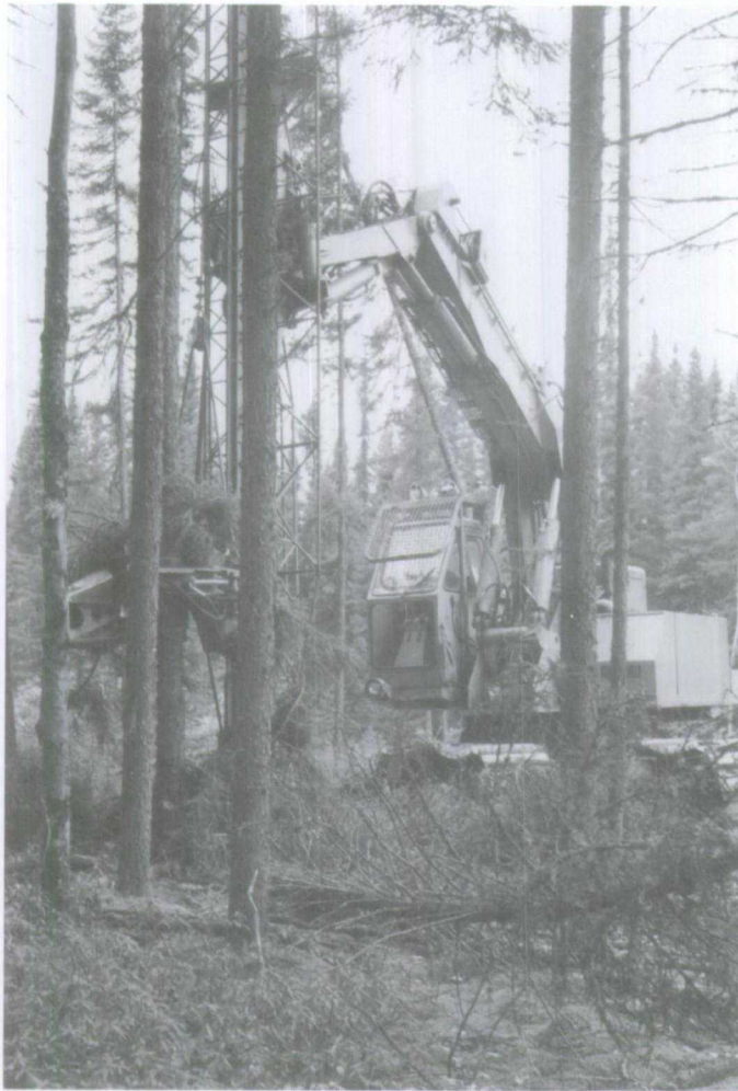
Figure 1.87 An early-model Beloit Harvester with a light lattice-type boom.
