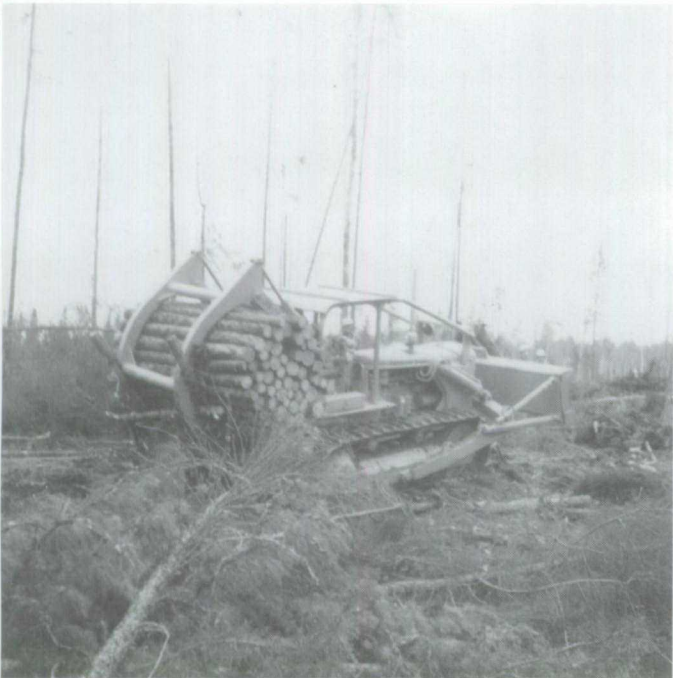
Figure 1.28 A Johnson skidder (in summer) forwarding a pile of eight-foot wood to the truck road.
