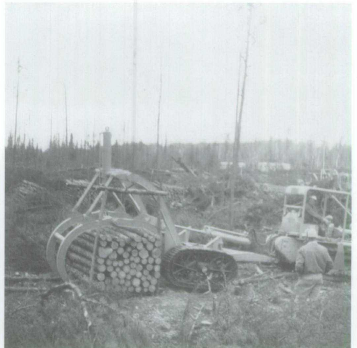
Figure 1.30 An Anderson Woodhawk (in summer) picking up a cord pile of 8-foot wood. Note that the piles have crib frames at each end of the pile instead of one frame at the centre of the pile.
