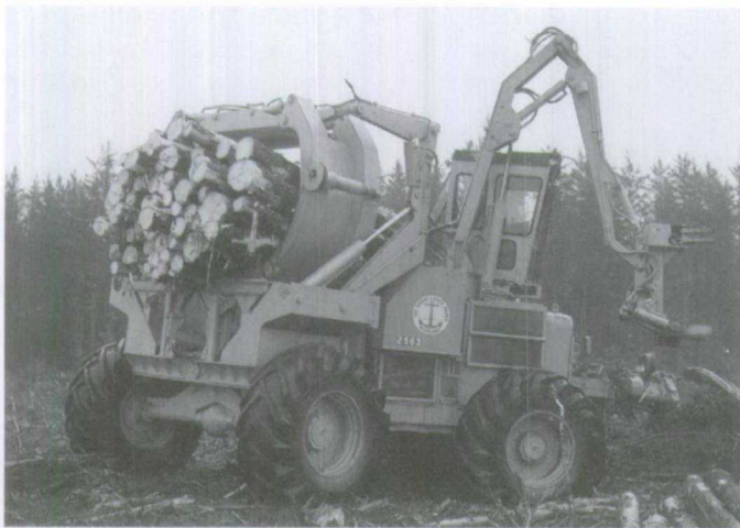
Figure 1.133 The loaded Larson Shortwood Harvester travelling to roadside landing. Final design of the cradle is essentially a large hydraulically operated grapple.
