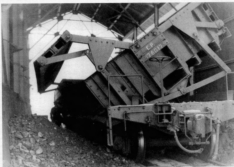
Figure 41. RAILCAR WITH COARSELY CRUSHED ORE AT COMINCO'S SULLIVAN CONCENTRATOR A rail car dumps its load of coarsely-crushed ore in 1938. (B.C. Archives)
