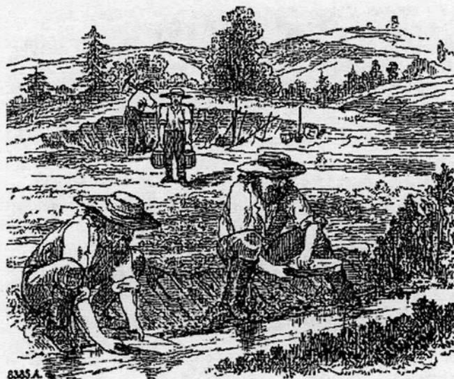
Figure 1. THE PAN Notwithstanding its ubiquitous use as the symbol of the rush era, the gold pan was rarely used for mining on an extensive scale. It remained an excellent prospecting tool, however, as well as an accurate way of estimating the relative richness of a particular deposit. 34 (from Egleston, Metallurgy )
