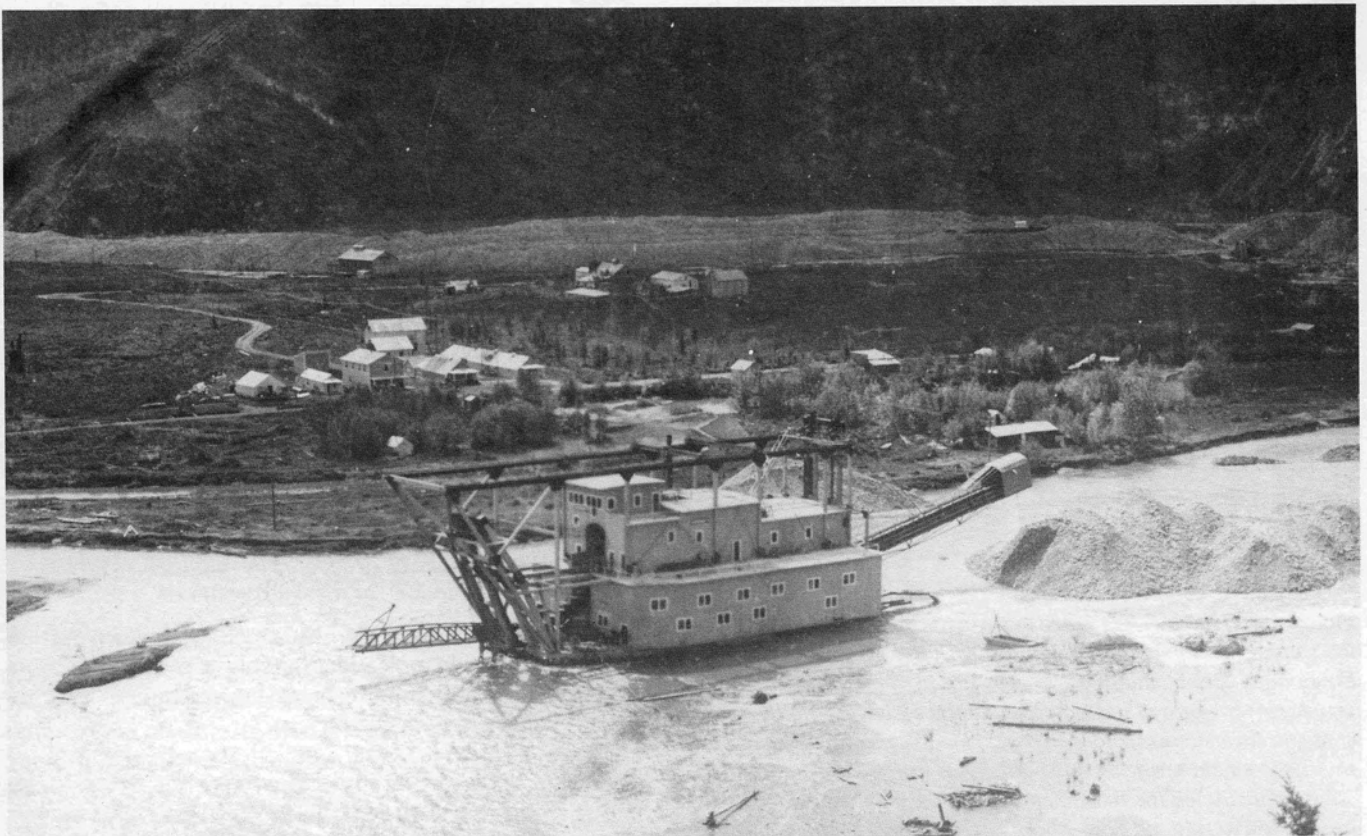
Figure 22. DREDGE NO.4 IN THE KLONDIKE RIVER, JUNE 14, 1914 The photograph of No. 4 Dredge on the Klondike River in the summer of 1914 indicates their method of working as well as their considerable environmental impact. (Yukon Archives)
