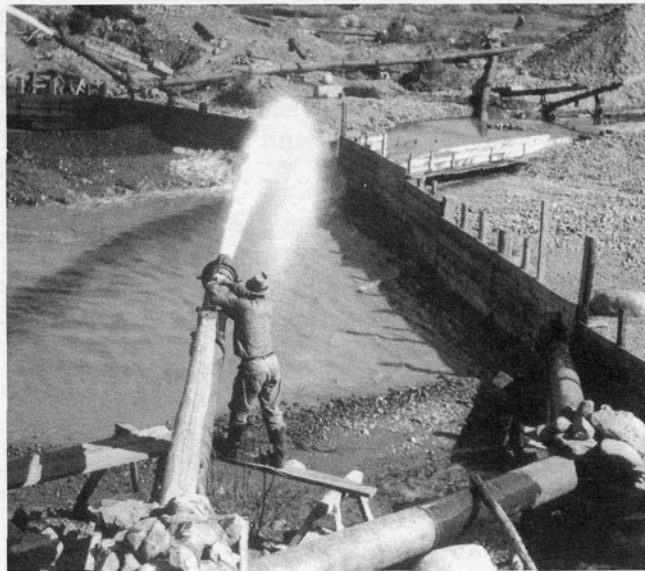
Figure 20. MCRAE-ACHESON HYDRAULIC OPERATION, PINE CREEK As placer mining shifted in focus and attempted to treat lower grade deposits, mechanization and economies of scale assumed far greater significance. Hydraulicking was developed in California in the 1850s and used powerful jets of water to blast gold-bearing gravels. It was relatively late in coming north, although ultimately it became a significant activity in the post-rush era in British Columbia. 9 Taken in the 1920s, this photo reveals the more extensive hydraulic activity in the Stikine region of northwestern British Columbia. (B.C. Archives)
