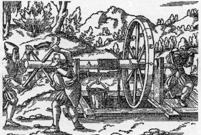
Figure 10. MINERS WORKING A CAPSTAN Although the Cariboo's shafts and waterwheels reflected a reasonably sophisticated grasp of engineering, nothing in the region would have been unfamiliar to a well-read sixteenth-century mining engineer in Europe. Compare the bucket and capstan in Figure 9 with those in the woodcut from Agricola's De Re Metallica , first published in 1556. (Agricola)
