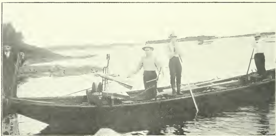
No. 21. — Metering on the Ottawa River above Ottawa with a Haskell current meter. The "fish tail" attachment keeps the meter truly in the direction of current.
