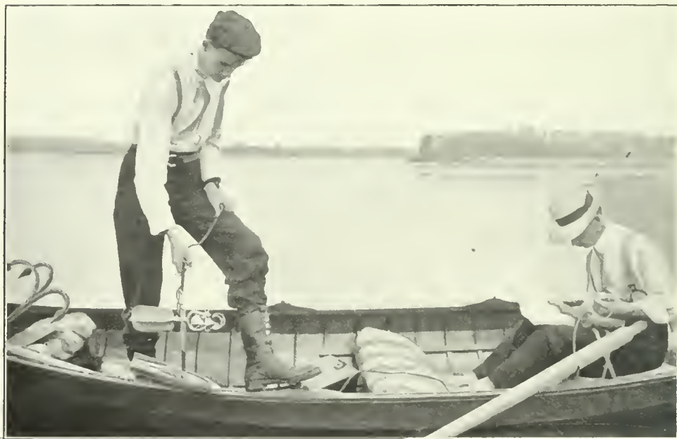
No. 19.—Metering with small Price current meter. The conical cups revolve fast or slow in response to the current, and revolutions are registered by an electric recorder, the time being taken by stop watch.
