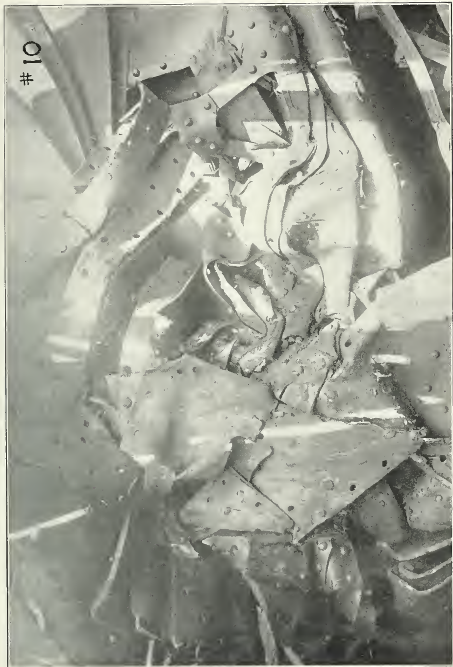
10. Shows the complete chaos to be seen at some points of the wreckage. This view is interesting only as an indication of the magnitude of the forces at work during the catastrophe. Even in this distorted mass there is no evidence of poor material.
