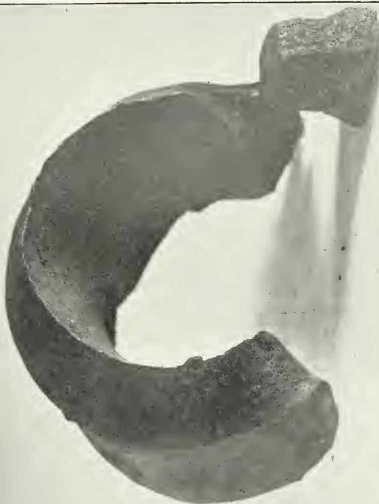
16. Shows a fragment of \frac{3}{4} " plate torn, sheared and bent.
