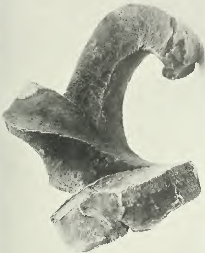
15. Shows a fragment of \xi'' plate torn, sheared and bent.
