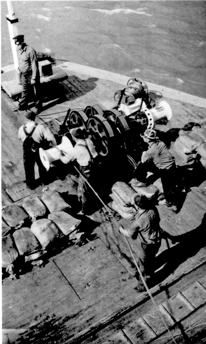
79 SS Klondike No. 2 lining through Five Finger Rapids. The cable was picked up with a pole and wrapped around the winch drum. Power was then applied and the boat pulled itself through. (Photo by B. Lesyk.)
